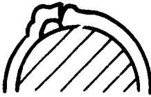
Buckling of Oxide on a Convex Surface
