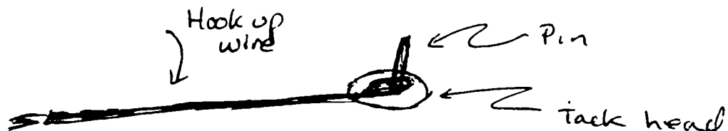
Figure 7 Wrapping the hook-up wire around the pin of a thumbtack
