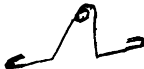
Figure 6 Bending the 'U' into the end of the paper clip to complete the coil support
