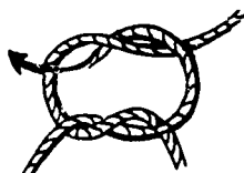
SQUARE KNOT Use to tie two light lines of the same size together. (Be sure that the line going into one side on top is going out on top as it comes back through--otherwise it's a granny knot and won't hold!)
