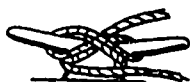
FIGURE EIGHT ON A CLEAT Use to tie to a cleat. (Make sure the line is wrapped around the base of the cleat first.)
