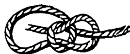
BOWLINE (pronounced bölyn) Use to tie a non-slip loop at the end of a line. The bowline does not jam and can be untied.
