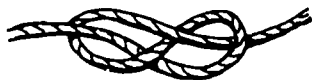
FIGURE EIGHT Use to keep the end of a line from unraveling or as something to hold onto.
