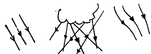
rectilinear light, coming from one direction: shadows can be formed. rectilinear, but diffuse light: no shadows will be formed. non-rectilinear light-propagation.
