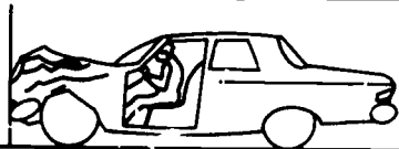
Within 1/10 of a second the car has come to a stop, but the person is still moving forward.
