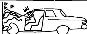
1/50 of a second after the car has stopped, the unbelted person slams into the dashboard or windshield. This is the human collision.
