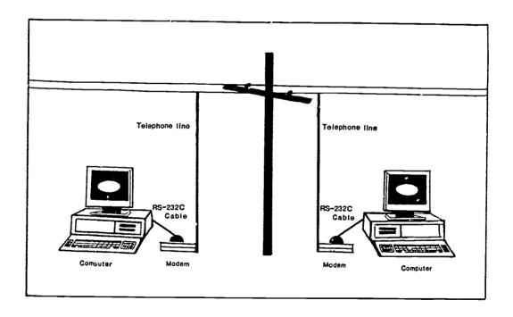
Fig. 1. This illustration identifies the components of the telecommunications process: a microcomputer, a modem, telephone lines, and an RS-232C cable.
