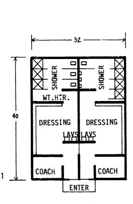
This 1,200 sq.ft. plan is intended to be constructed of 8" concrete block bearing walls and standard wood roof rafters.
