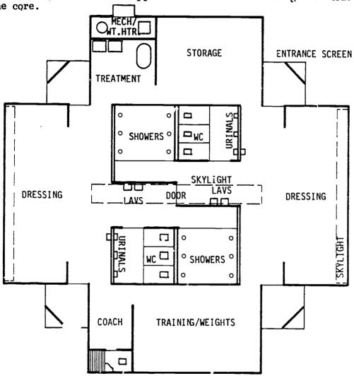
The concept is represented by two intersecting 2 X 4 rectangles. Any unit of measure can be assigned to the rectangles. The size of the rectangles is limited only by the required square footage. The plan diagram illustrates the 2 X 4 rectangles containing approximately 2,700 square feet if a value of 30' X 60' is assigned to each of the intersecting rectangles.
