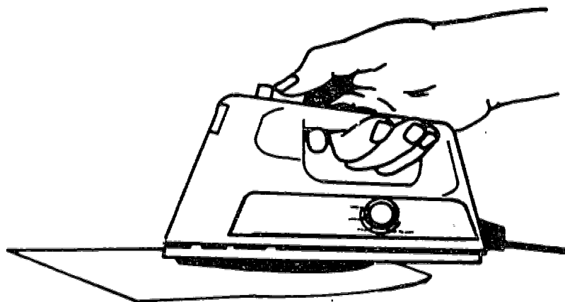
Figure C-4-11 Heating the Object with a Steam Iron
