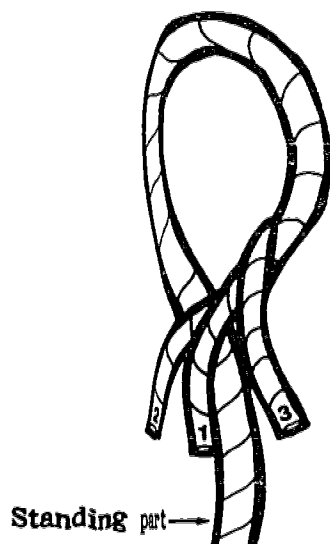
Figure F-1-7 Part A. Eye-Splice Strands Separated and Eye Tied Off
