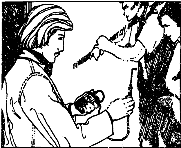
FIGURE 8. Measuring the surface temperature of a painting with the Aotek thermometer. Extreme care is needed so as not to damage the surface of the painting with the probe.
