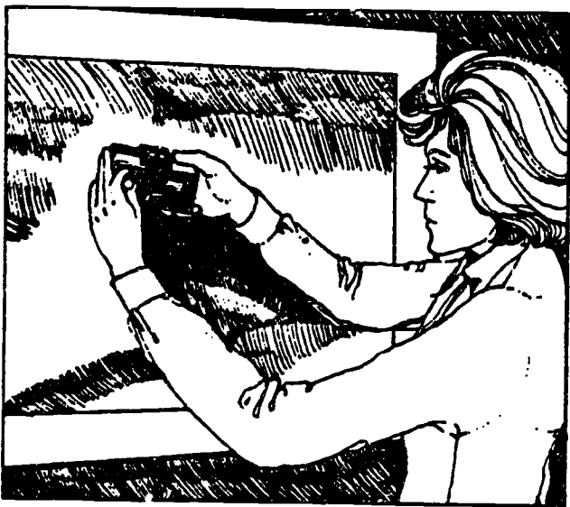
FIGURE 12. Measuring ultraviolet radiation incident on a painting with the Crawford Type 760 monitor.
