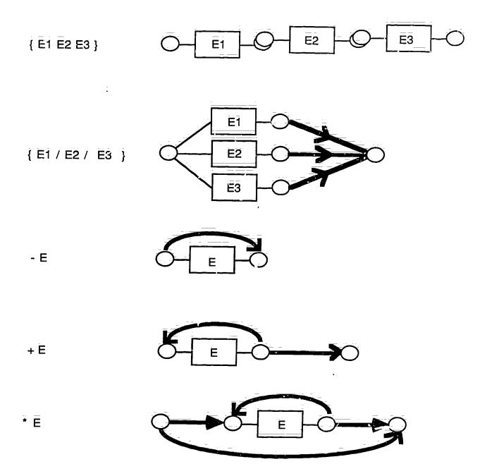
Network Implementation of HGSL constructs. Figure 1 Boxed "E" and thin arrows are the previously constructed net of the arbitrary expression E.
