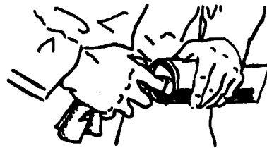
Fig 1-48. Wiping joint surfaces with a rag.
