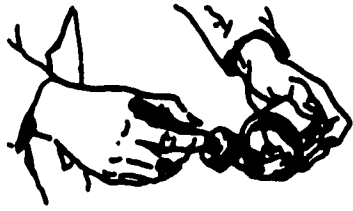
Fig 1-51. Applying cement to fitting socket.
