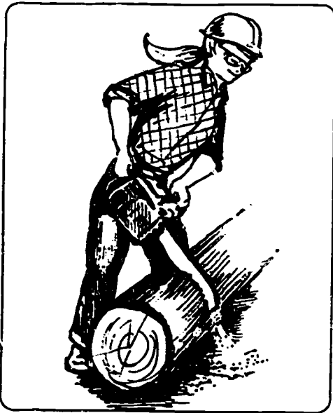
Figure 3.13. Keep legs out of the path of the saw. Brace the back of the saw against the upper leg to increase control.
