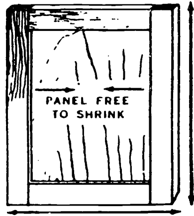
STRENGTH IN BOTH LENGTH AND WIDTH OF FRAME
