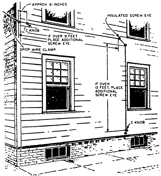
Figure 3-24. Drop wire run on frame building.
