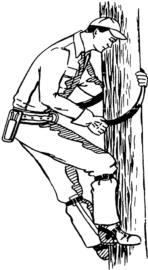
Figure 2-28. Transferring the safety strap.
