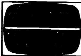
D NO VERTICAL DEFLECTION
