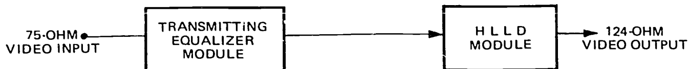
Figure 2-2. Balanced line driver block diagram.
