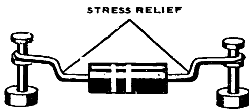
Figure 2-43. Typical stress reliefs bend in part leads.
