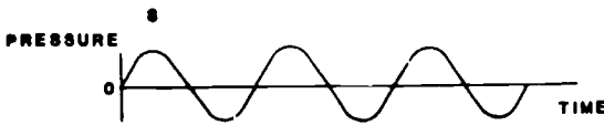
Figure 3-1 Sound waves illustrated in sine wave form. Line A shows a single cycle, line B is a continuous cycle sound wave.
