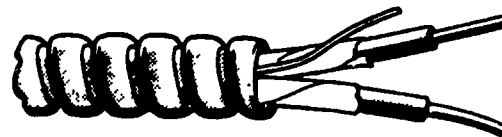
METALLIC ARMORED CABLE. TWO-WIRE CABLE WITH BARE GROUND
