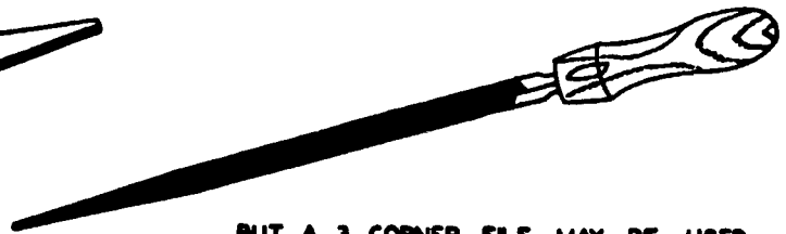
BUT A 3 CORNER FILE MAY BE USED ON LARGER BITS.
