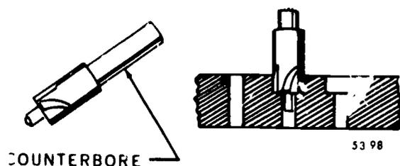
Figure 98. Counterbore and counterbored hole.
