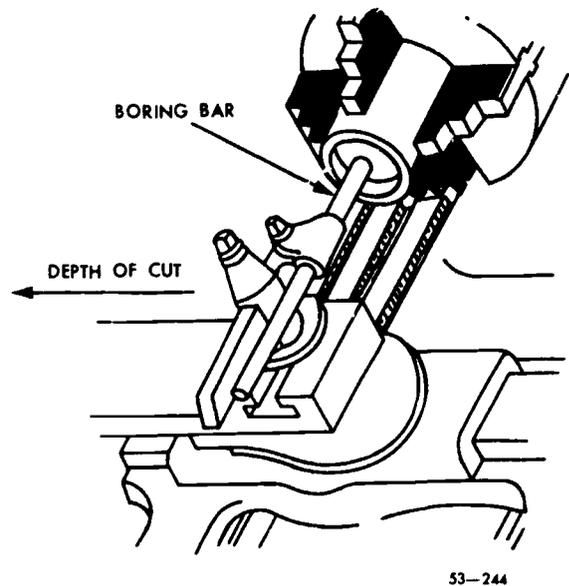
Figure 109. Boring in the lathe.
