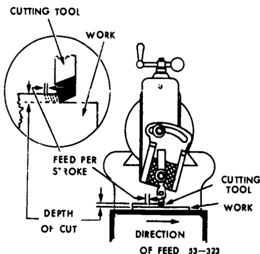
Figure 4. Shaper feed and depth of cut.
