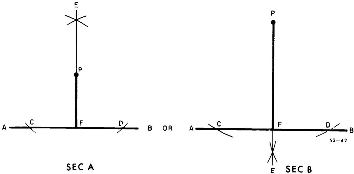
Figure 42. Erecting a perpendicular through a point off a line.
