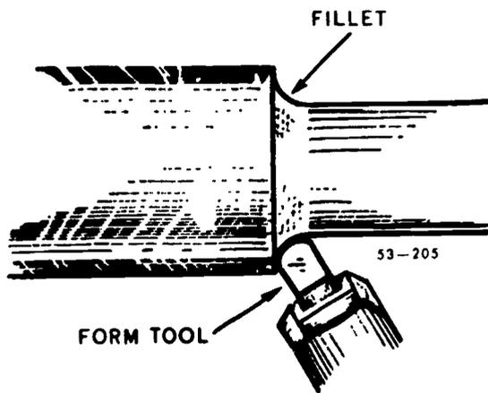
Figure 70 Machining a filleted corner.
