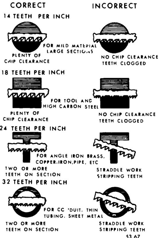
Figure 67. Section of pitch.
