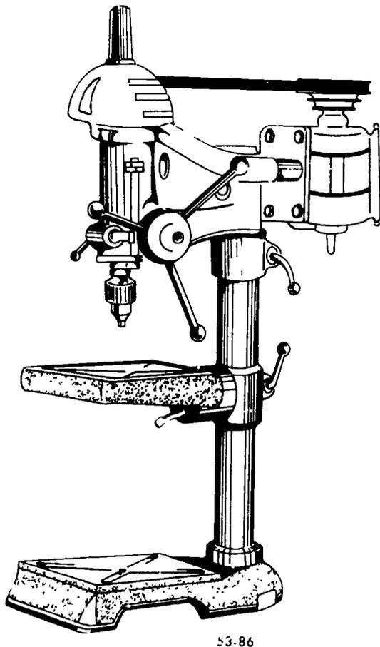
Figure 86. Bench-mounted drill press.
