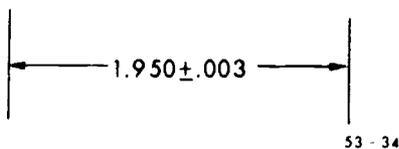
Figure 34. Equal bilateral tolerance.
