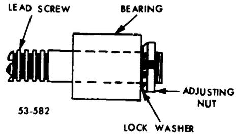
Figure 151. Lead screw end play adjustment.
