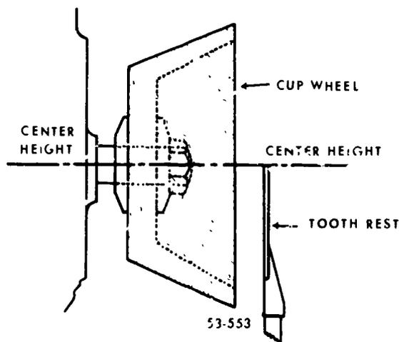
Figure 115. Alinement of tooth rest with axis of cup wheel.
