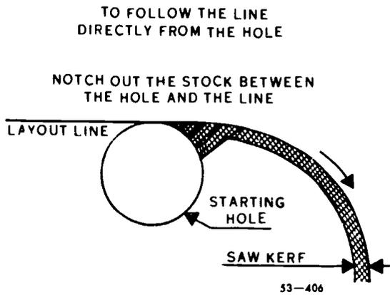
Figure 87. Sawing tangent to a starting hole
