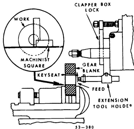
Figure 61. Alineing gear and positioning extension toolholder.
