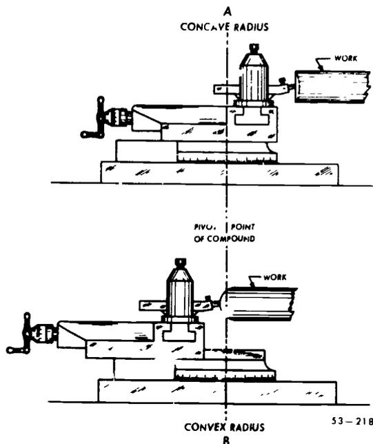
Figure 83. Machining a radius with the compound rest.
