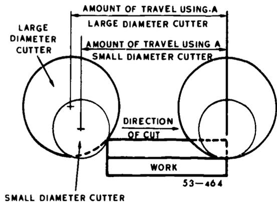
Figure 33. Cutter diameter selection.
