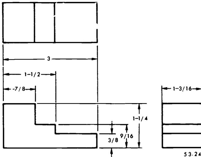
Figure 24. Dimensioning methods.
