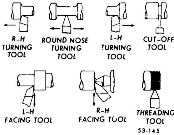
Figure 10. Cutting tool shapes.
