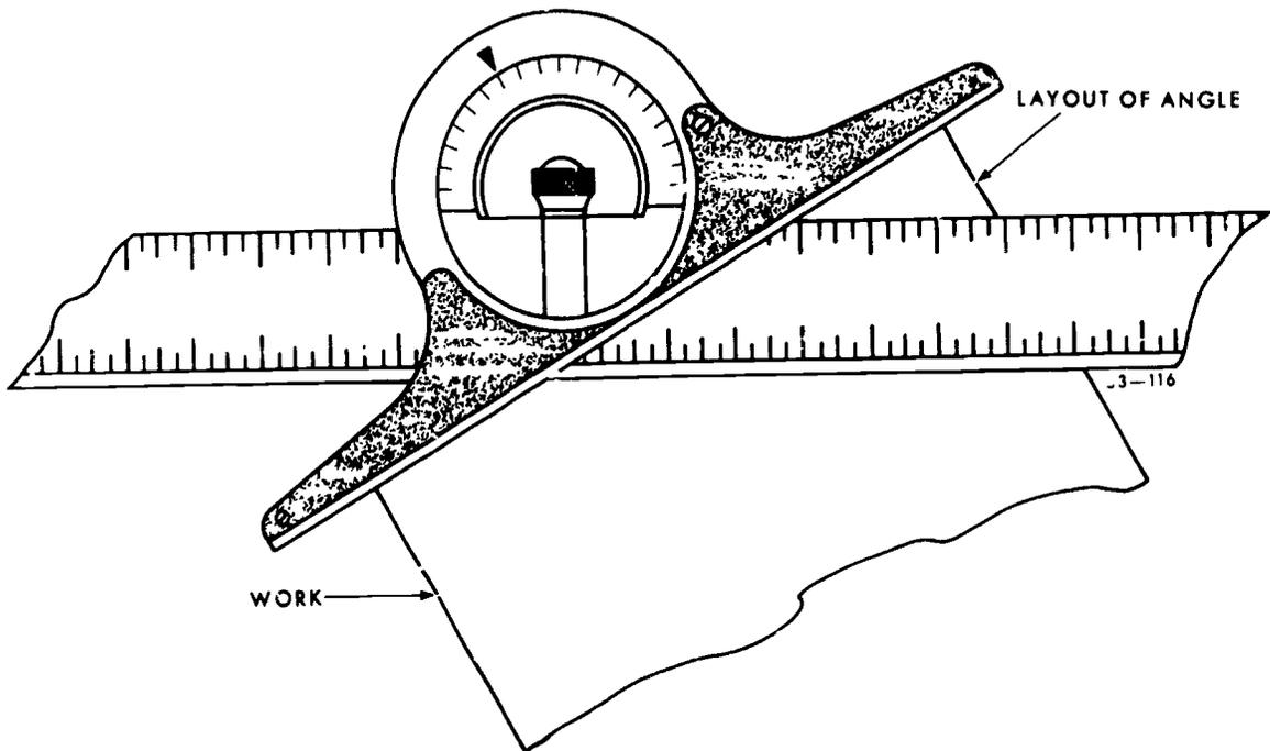
Figure 116. Use of protractor head.
