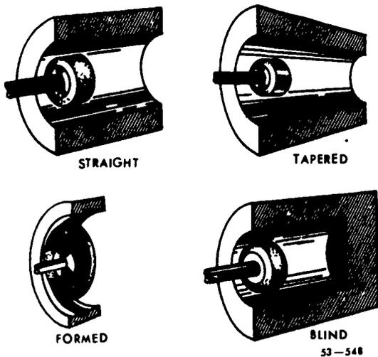
Figure 110. Typical internally ground surfaces.
