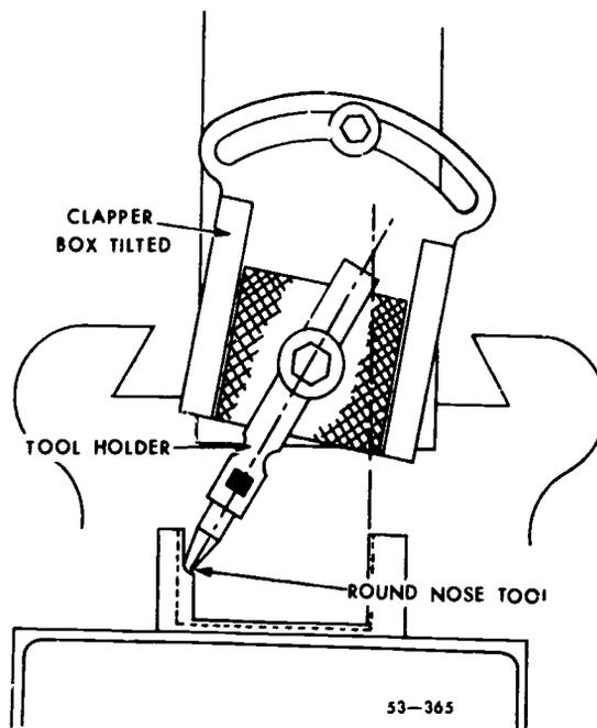
Figure 45. Tilting clapper box for down cutting
