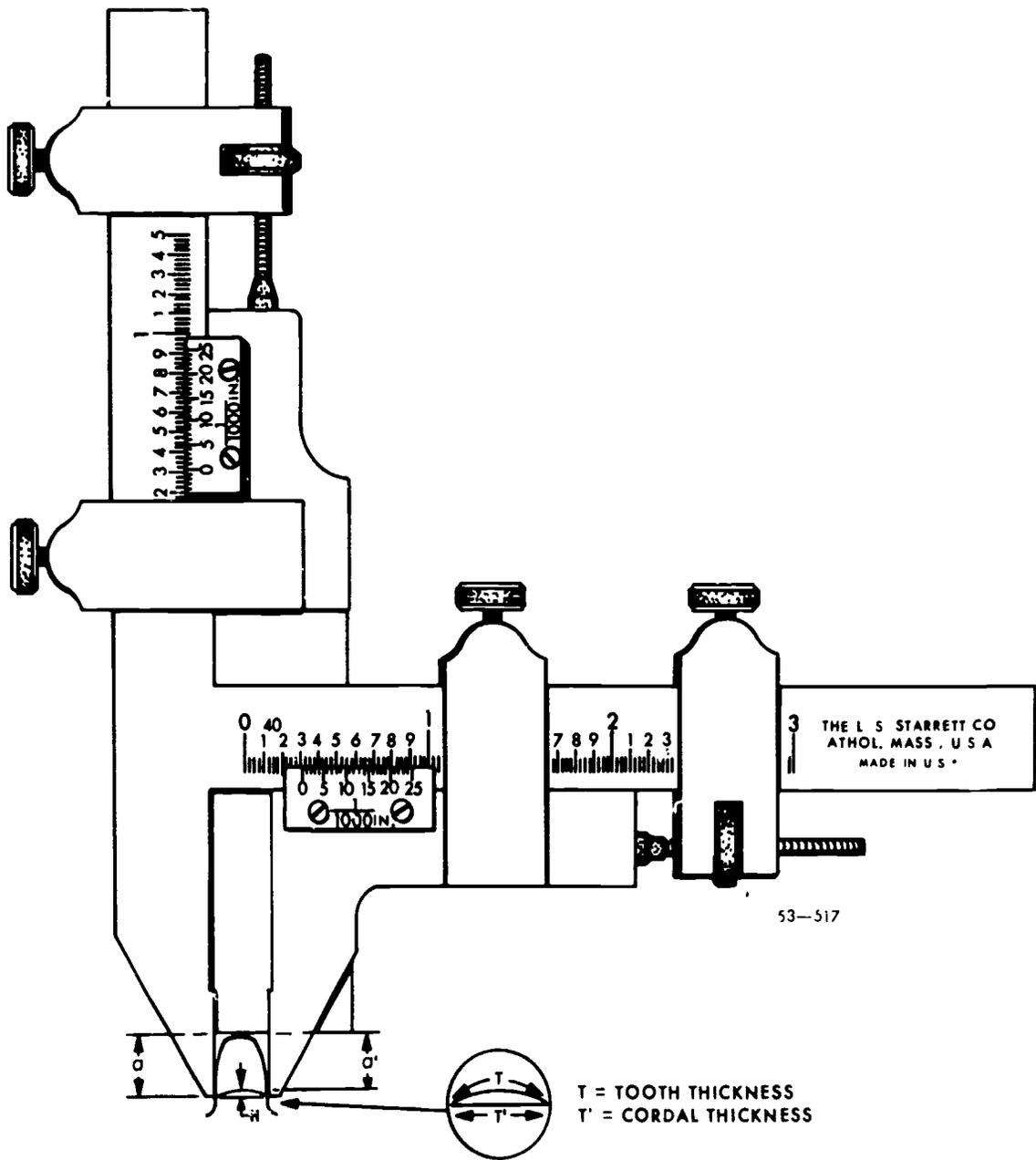
Figure 82. Vernier gear tooth caliper.
