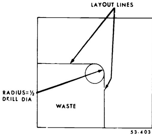
Figure 83. Drilled corner hole.
