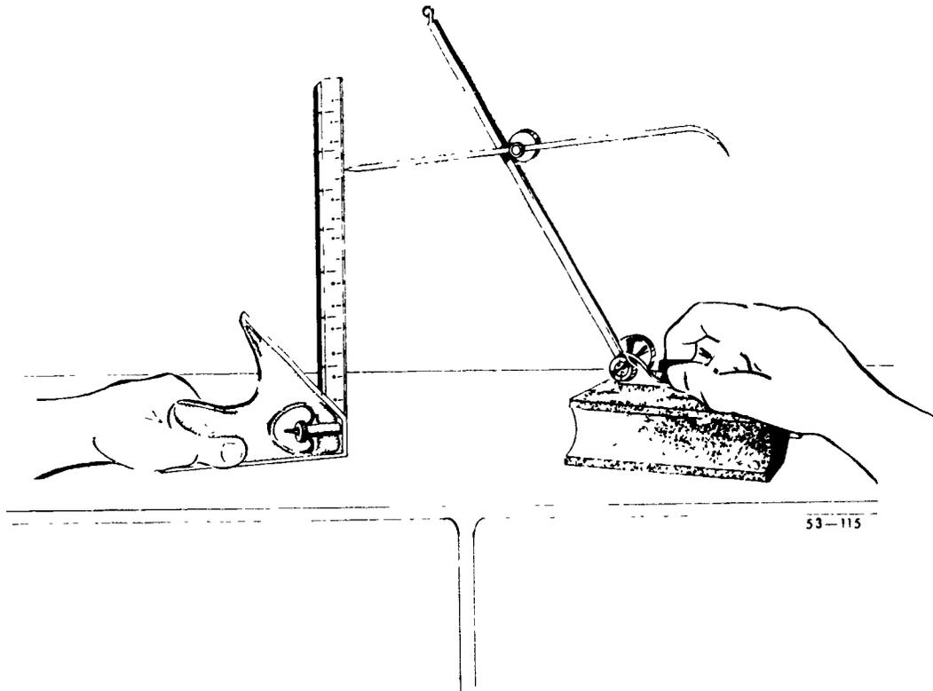
Figure 115. Setting surface gage to square head.
