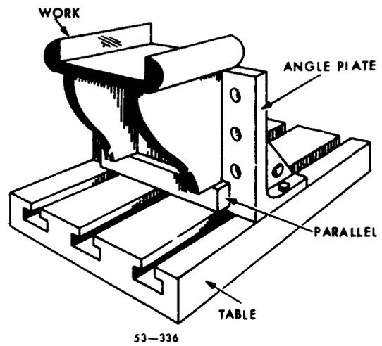
Figure 17 Nonadjustable angle plate.
