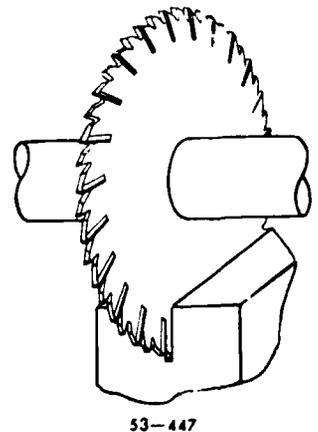
Figure 16. Slitting saw with staggered teeth.
