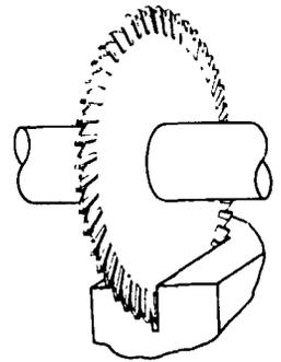
Figure 15. Slitting saw with side teeth.
