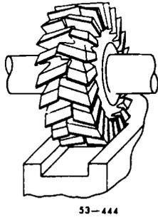
Figure 13. Interlocking teeth side milling cutter.
