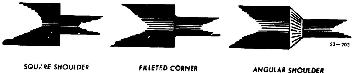
Figure 68. Three common types of shoulders.
