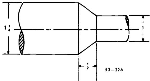
Figure 91. Dimensions of a taper.
