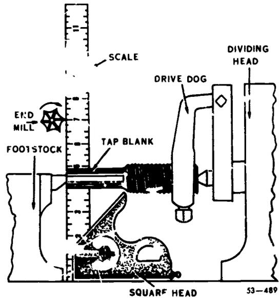
Figure 58. Alining the work and cutter.
