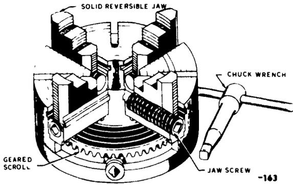
Figure 28. Four-jaw combination chuck.
