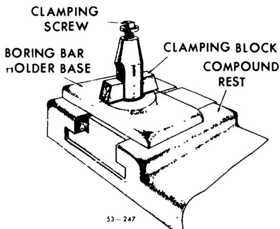
Figure 112. Use of the clamping block.
