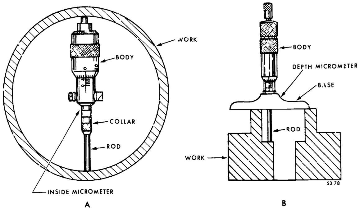
Figure 78. Inside and depth micrometers.
