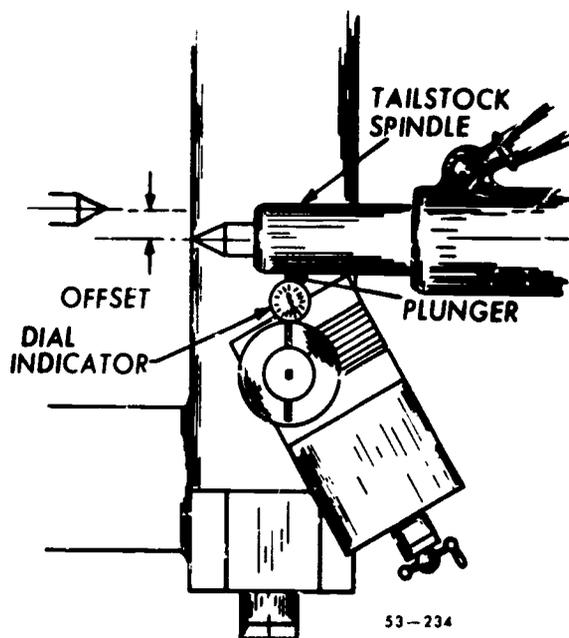
Figure 99. Measuring offset with a dial indicator.
