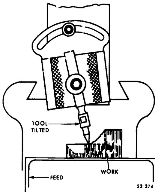
Figure 54. Roughing excess to one shoulder.
