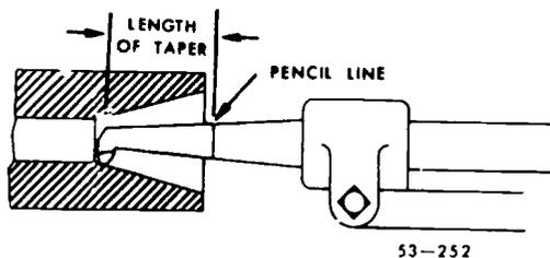
Figure 117. Marking boring bar.
