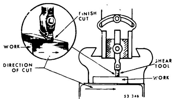
Figure 27. Cutting action of a shear tool.
