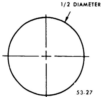
Figure 27. Dimensioning small diameters.
