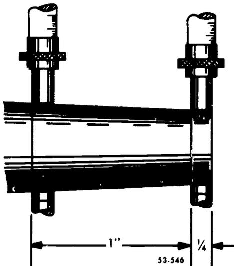
Figure 108. Measuring taper per inch (TPI).
