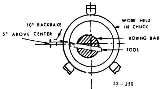
Figure 115. Boring tool position.
