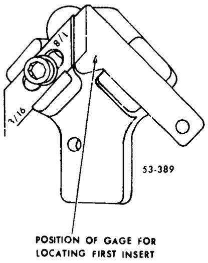
Figure 70 Installing left insert
