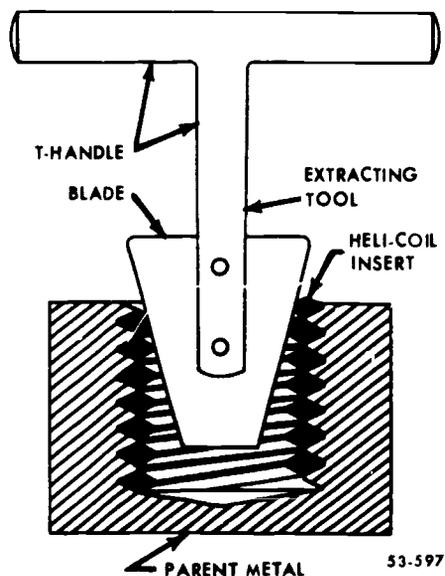
Figure 144. Heli-coil extracting tool.
