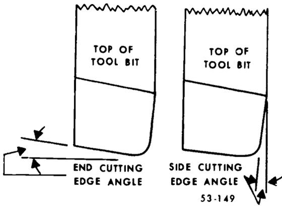
Figure 14. Cutting edge angles.
