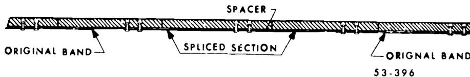
Figure 77 File band repair
