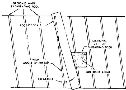
Figure 148. Checking side clearance of threading tool.
