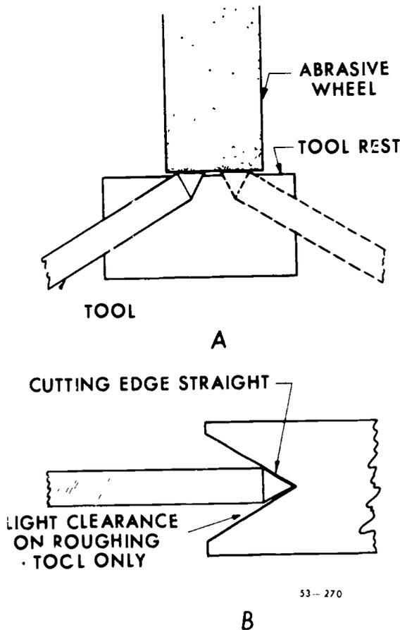
Figure 135. Grinding threading tool form.
