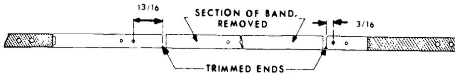
STEP III FIT SPLICE PART INTO PLACE AND RIVET SEGMENTS TO SPLICED SECTION
