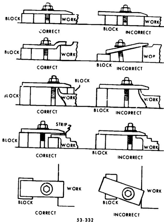
Figure 13. Clamping work.
