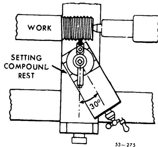
Figure 140 Position of compound rest.
