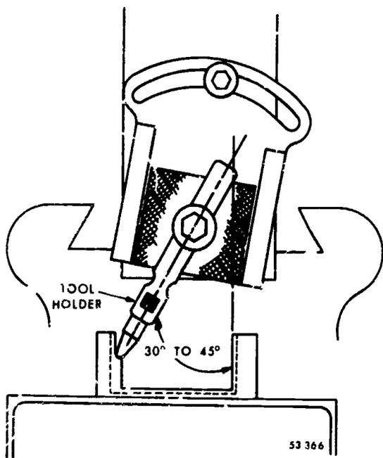
Figure 46. Positioning toolholder for internal vertical surfaces.
