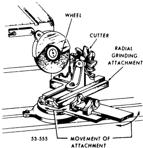
Figure 117. Radial grinding setup.
