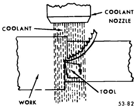
Figure 82. Application of coolant.
