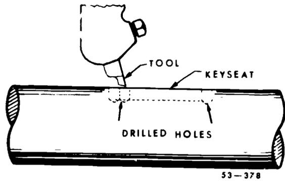
Figure 59. Keyseat slotting tool.
