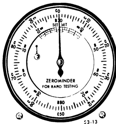
Figure 13. Dial face of a Rockwell hardness tester.
