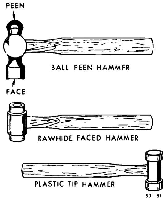
Figure 51. Hammers and mallets.
