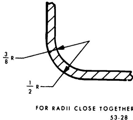
Figure 28. Dimensioning arcs and radii.
