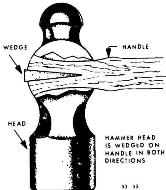
Figure 52. Securing head on handle.
