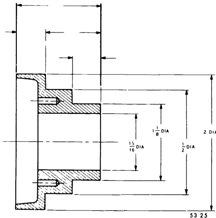
Figure 25. Dimensioning methods shown in profile.
