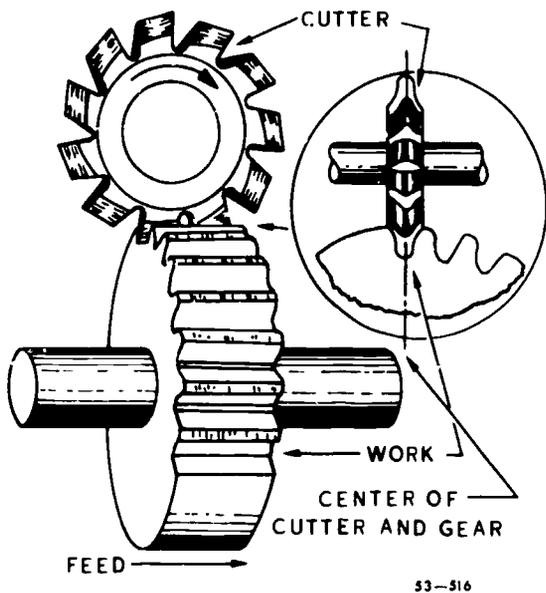
Figure 80. Milling a spur gear.
