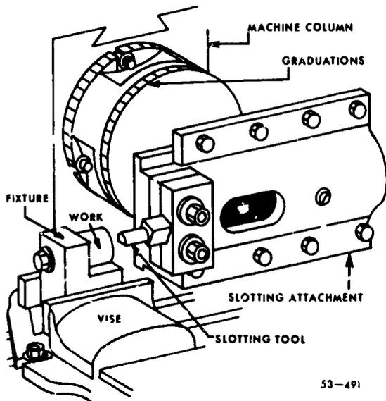
Figure 60. Slotting attachment.
