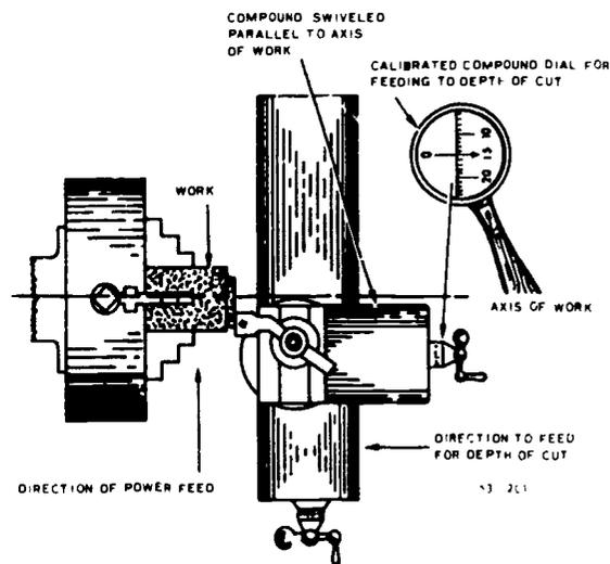
Figure 66. Facing work using the compound rest graduated collar.
