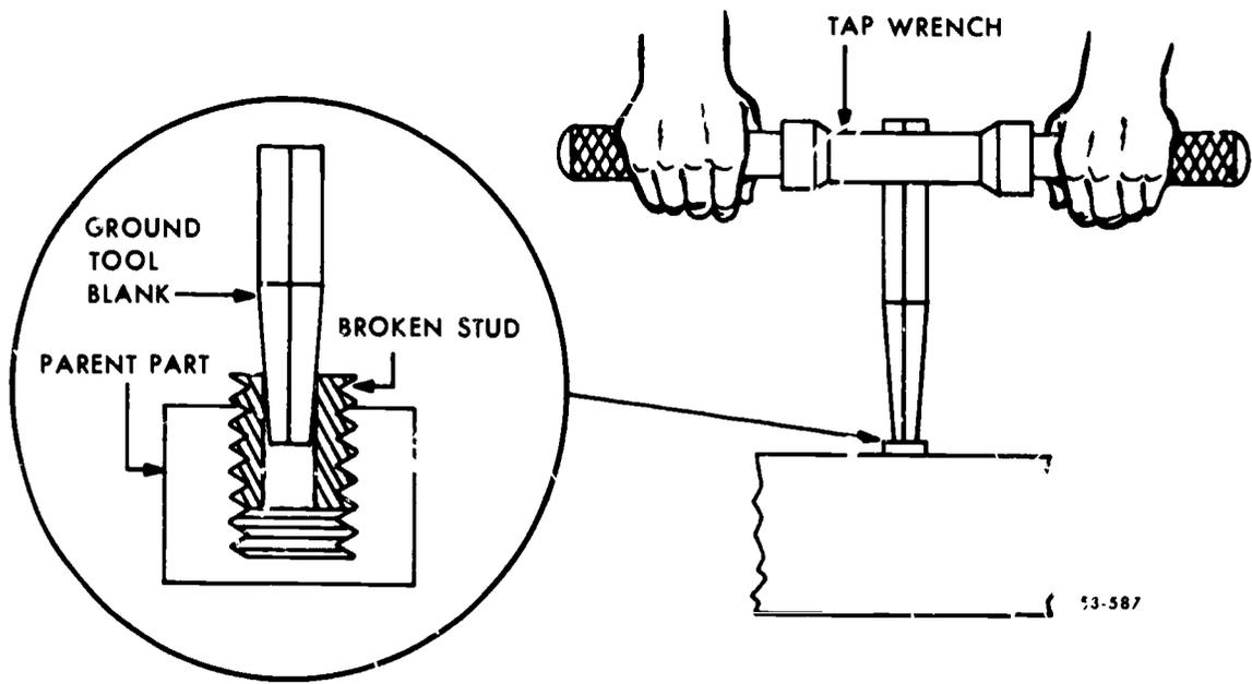
Figure 134. Ground tool type extractor.
