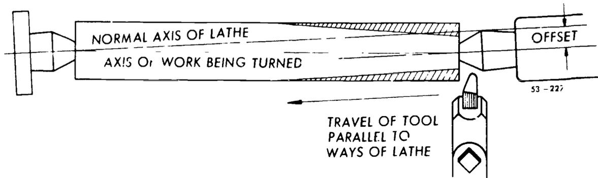
Figure 92. Effect of tailstock offset.
