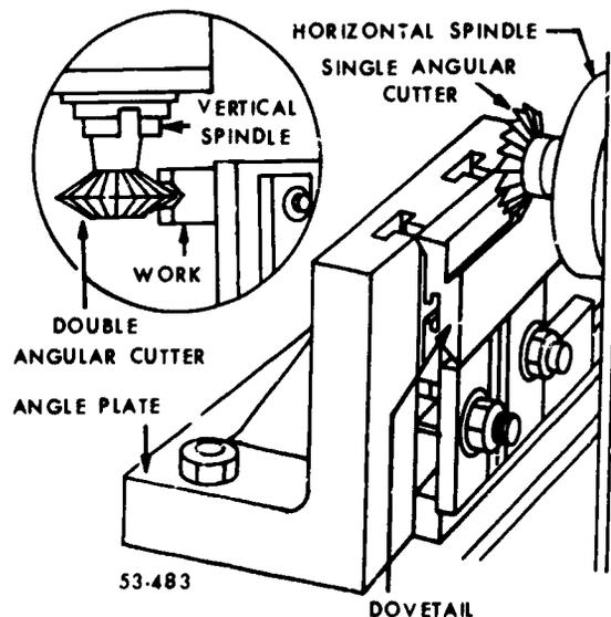
Figure 52. Angular milling.
