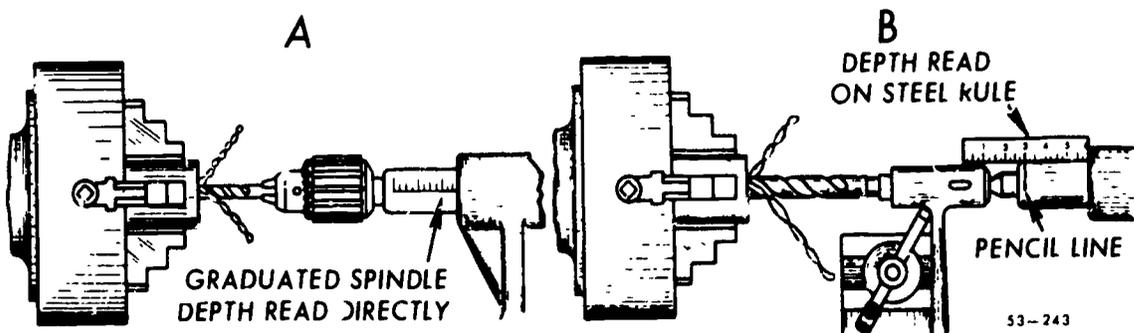
Figure 108. Measuring drill depth.
