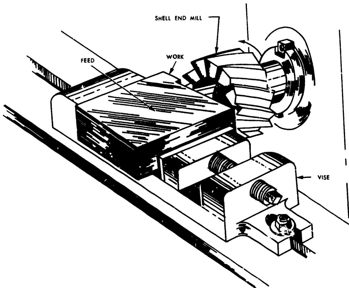
Figure 48. Face milling.
