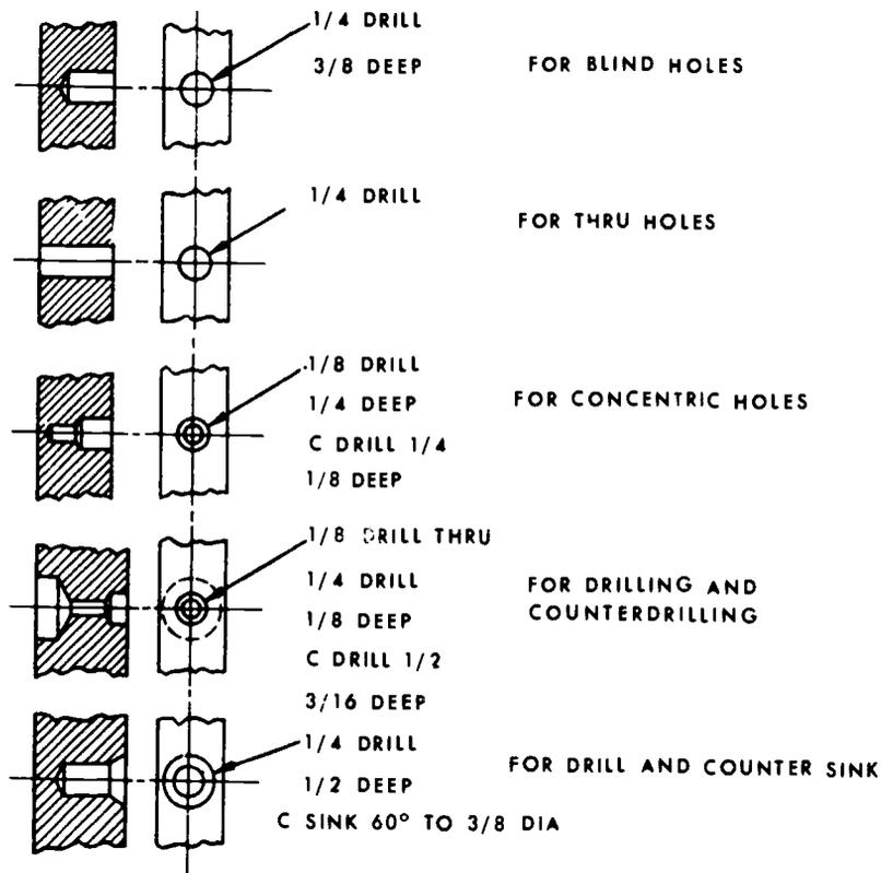
LENGTH OF DRILL POINT = DRILL DIA  $\times$  30043 FOR STD DRILL OF 118° INCLUDED ANGLE
