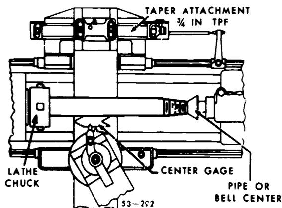
Figure 157. Pipe threading setup.
