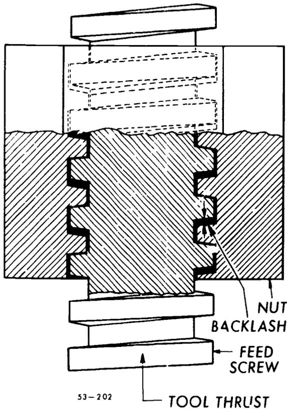
Figure 67. Backlash between feedscrew and nut.
