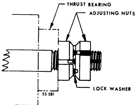
Figure 150. Crossfeed screw end play adjustment.
