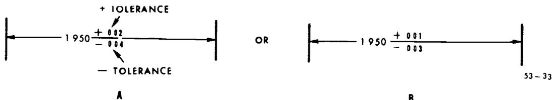
Figure 33. Unequal bilateral tolerance.
