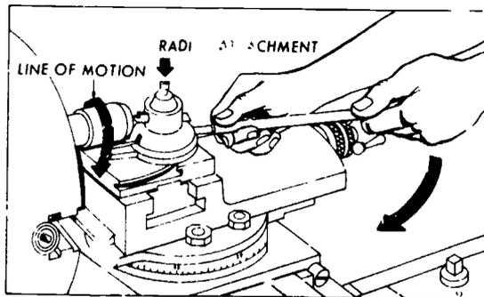
Figure 84. Radius turning attachment.
