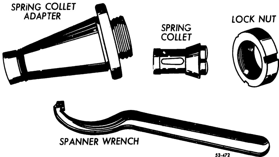
Figure 41. Spring collect chuck adapter.
