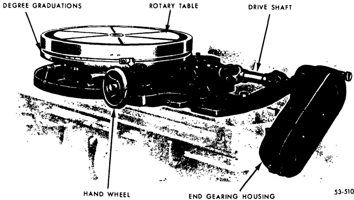
Figure 74. Circular milling attachment.
