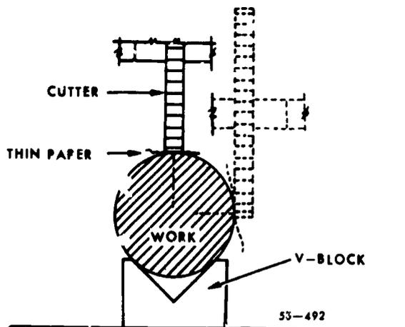
Figure 61 Alining cutter using a paper strip.
