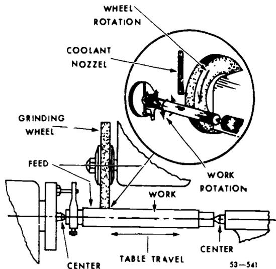
Figure 103. Cylindrical grinding.
