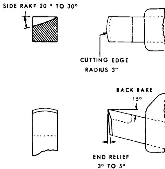
Figure 26. Shear tool for steel.
