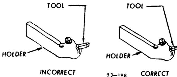
Figure 63. Cutting tool in toolholder.
