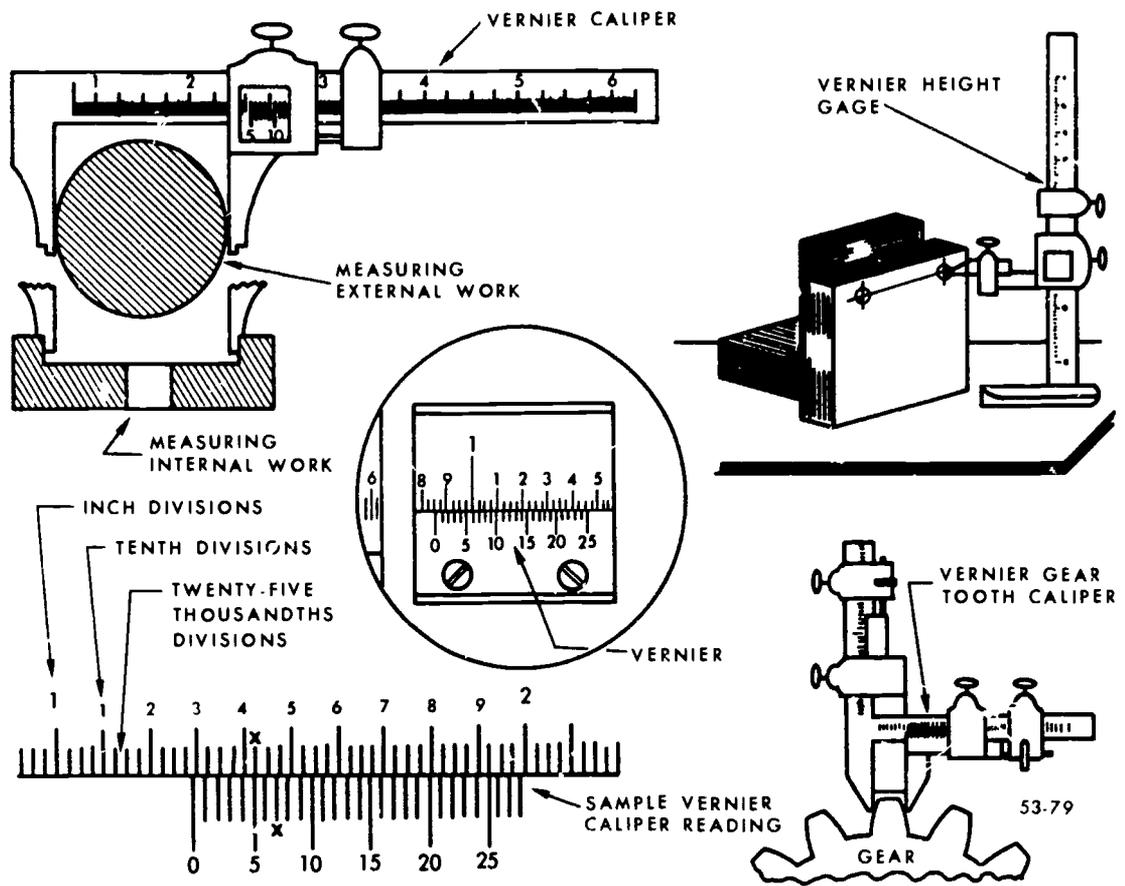
Figure 79. Vernier calipers and height gage.
