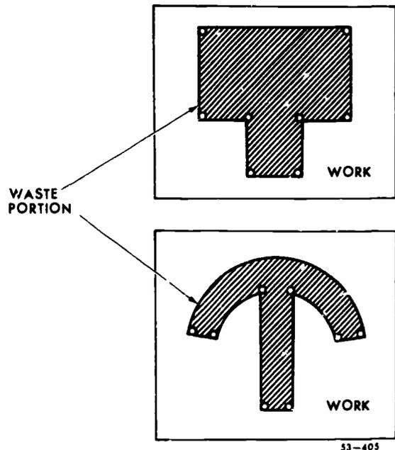
Figure 86. Internal contour.
