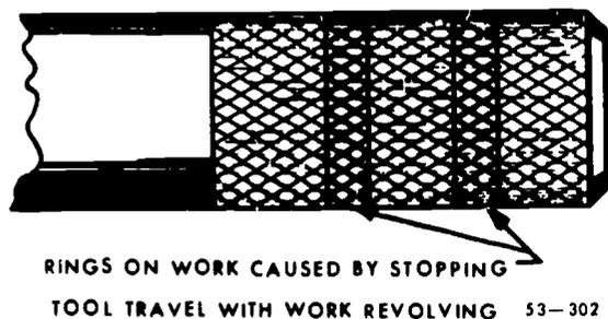
Figure 167. Rings on a knurled surface.
