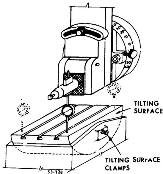
Figure 9. Alining tilting surface.
