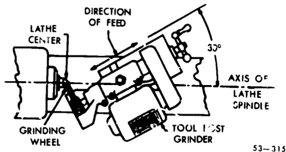
Figure 180. Grinding a lathe center.
