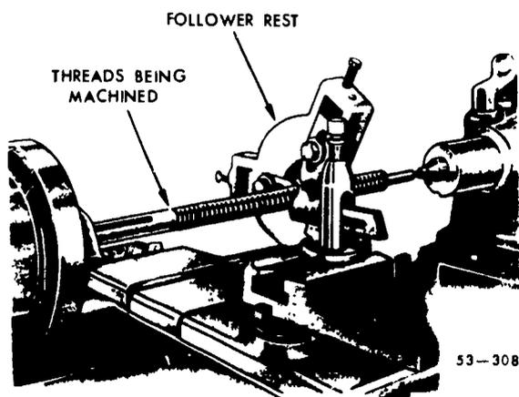
Figure 174. Follower rest used while threading.
