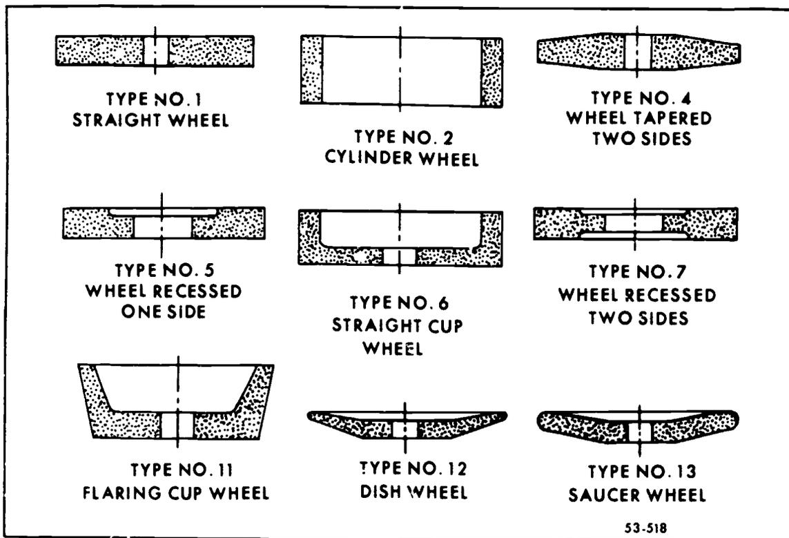
Figure 83. Standard grinding wheel shapes.
