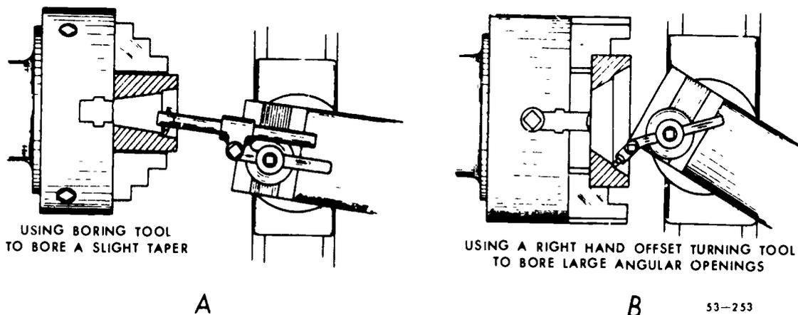
Figure 118. Boring short tapers.
