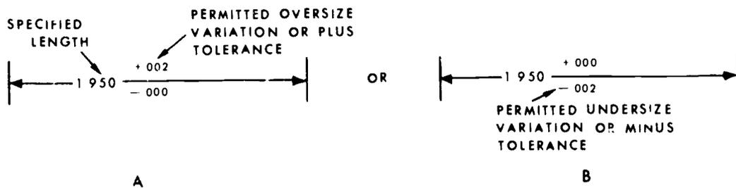
Figure 32. Unilateral tolerance.
