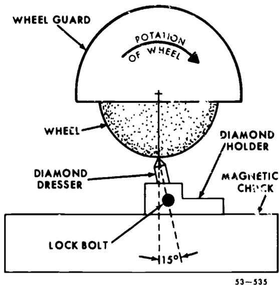
Figure 97. Surface grinder wheel dressing setup.
