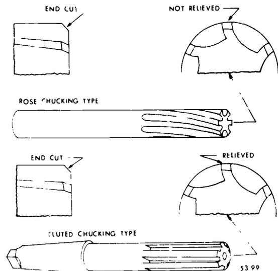
Figure 99. Machine reamers.
