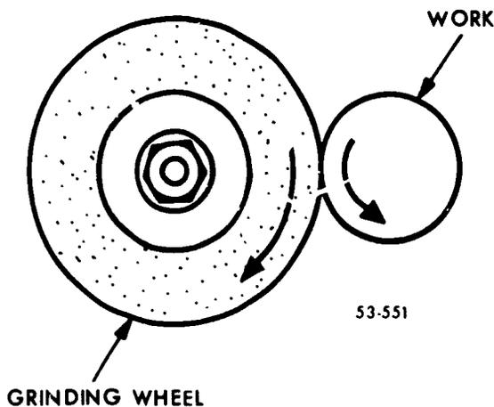
Figure 113. Wheel and cutter rotation for cylindrical grinding.
