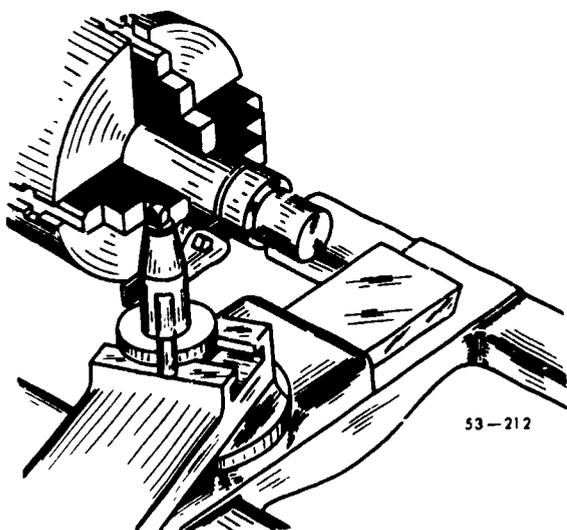
Figure 77. Parting setup.
