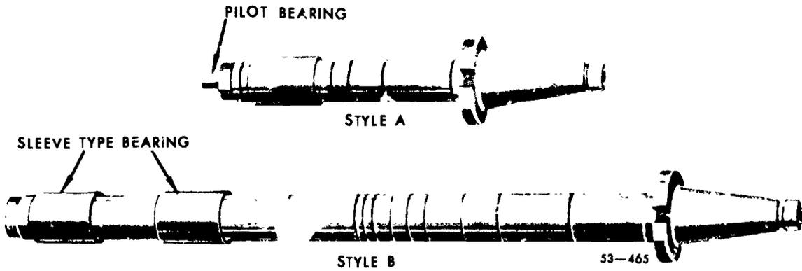
Figure 34. Standard milling machine arbors.
