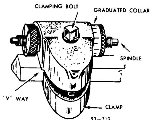
Figure 175. Micrometer carriage stop.
