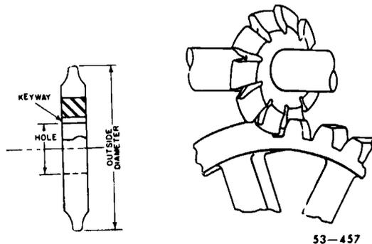
Figure 26. Involute gear cutter.
