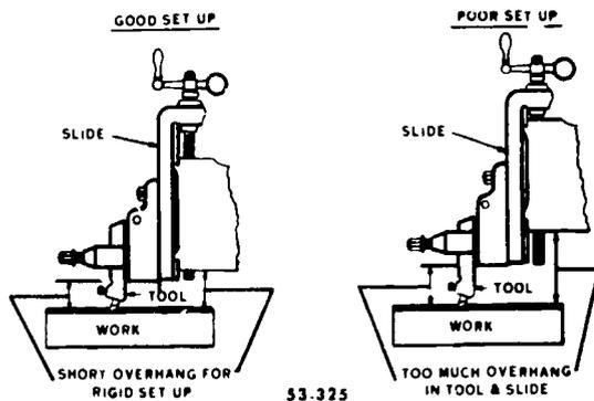
Figure 6. Tool and toolhead overhang.
