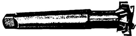
Figure 24. T-Slot cutter.
