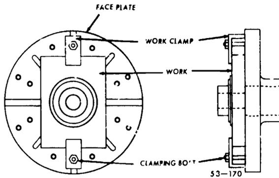
Figure 35. Work clamped on faceplate
