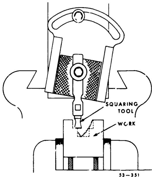
Figure 57. Machining a wide groove.
