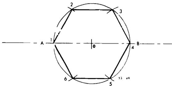
Figure 49. Constructing a regular hexagon.
