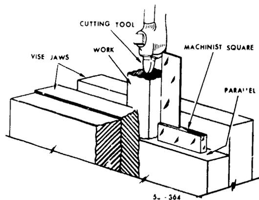
Figure 44 Positioning a short piece in the vise.
