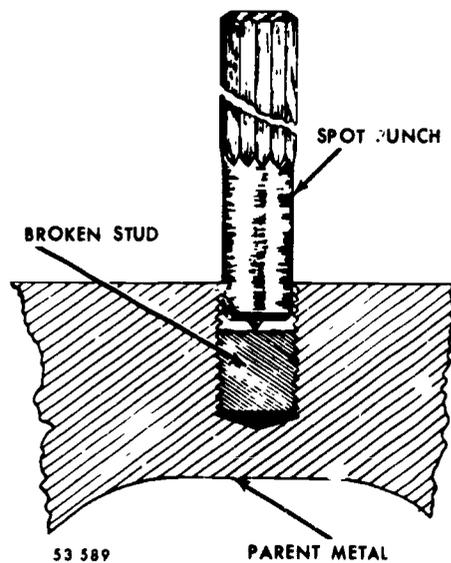
Figure 136. Spot punching a broken stud.
