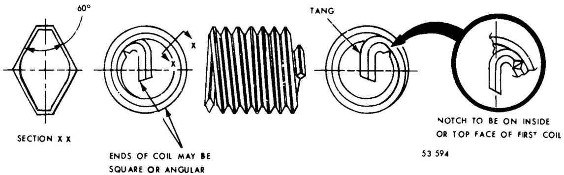
Figure 141. Diagram of a heli-coil insert.
