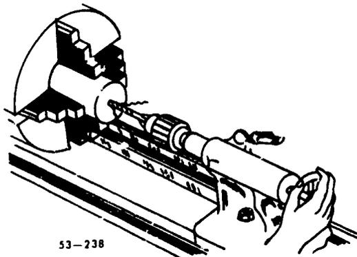
Figure 103. Feeding a drill into the work.
