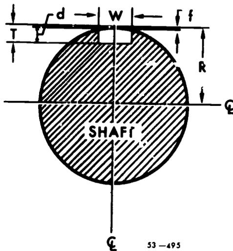
Figure 64. Keyseat dimensions for straight square key.
