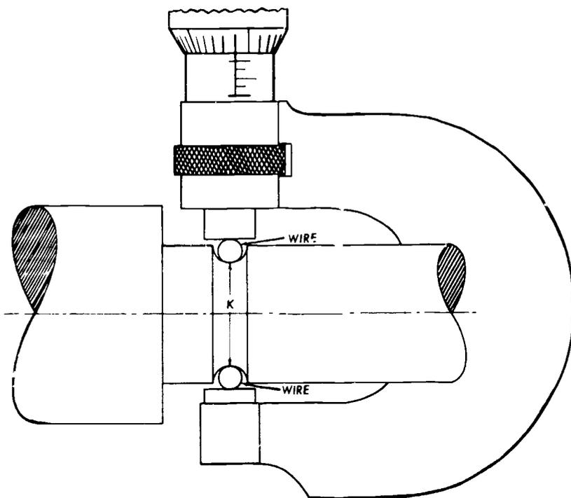
MICROMETER READING =  $K + 2(\text{WIRE DIA})$
