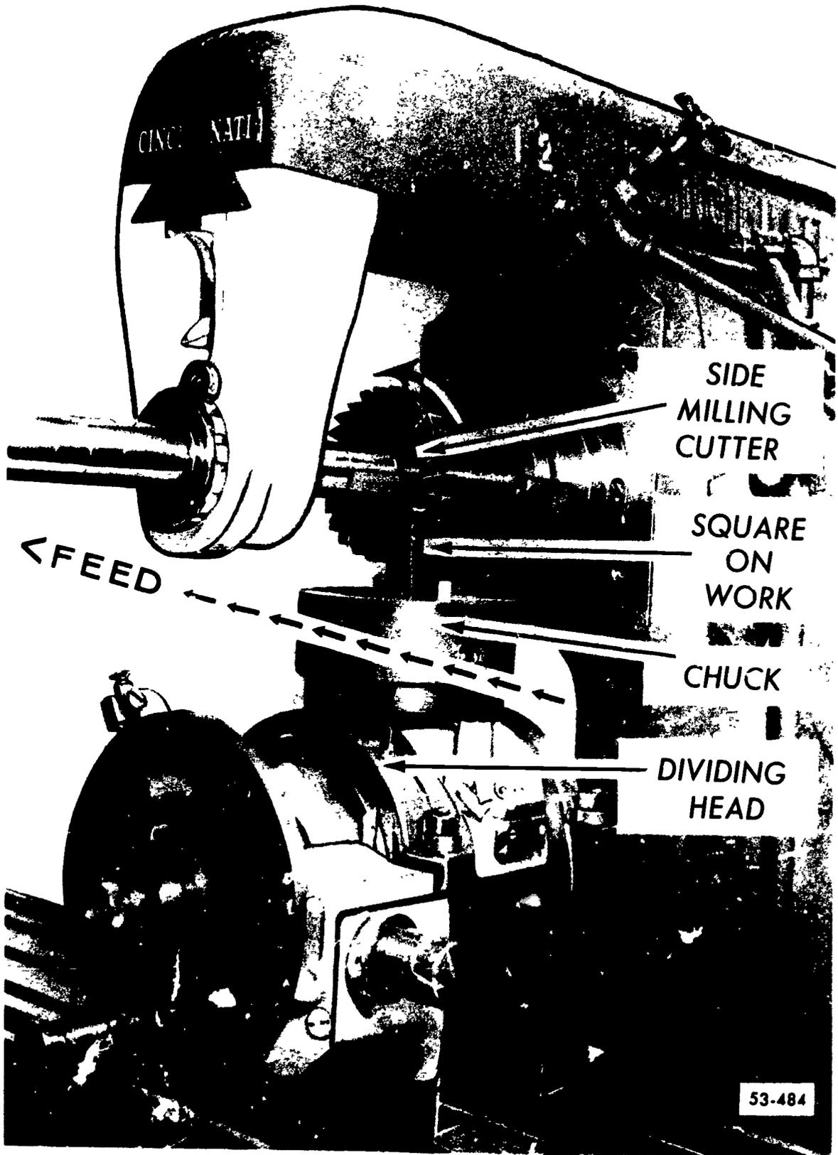
Figure 53. Milling a square on work held vertically.
