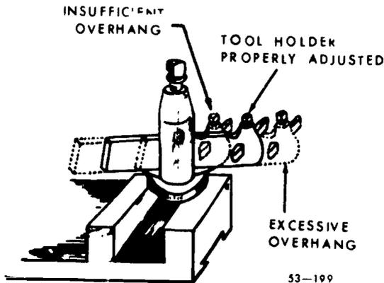
Figure 64. Toolholder overhang.
