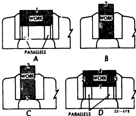
Figure 47. Machining sequence to square a block.
