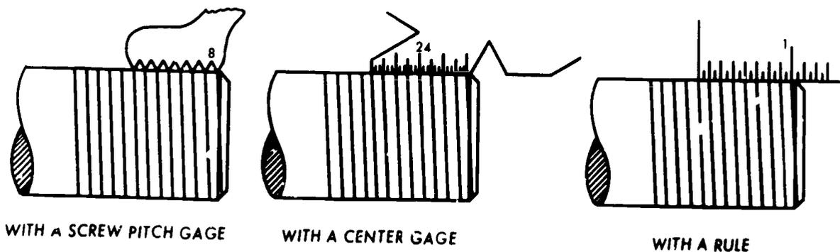
Figure 147. Checking thread pitch.
