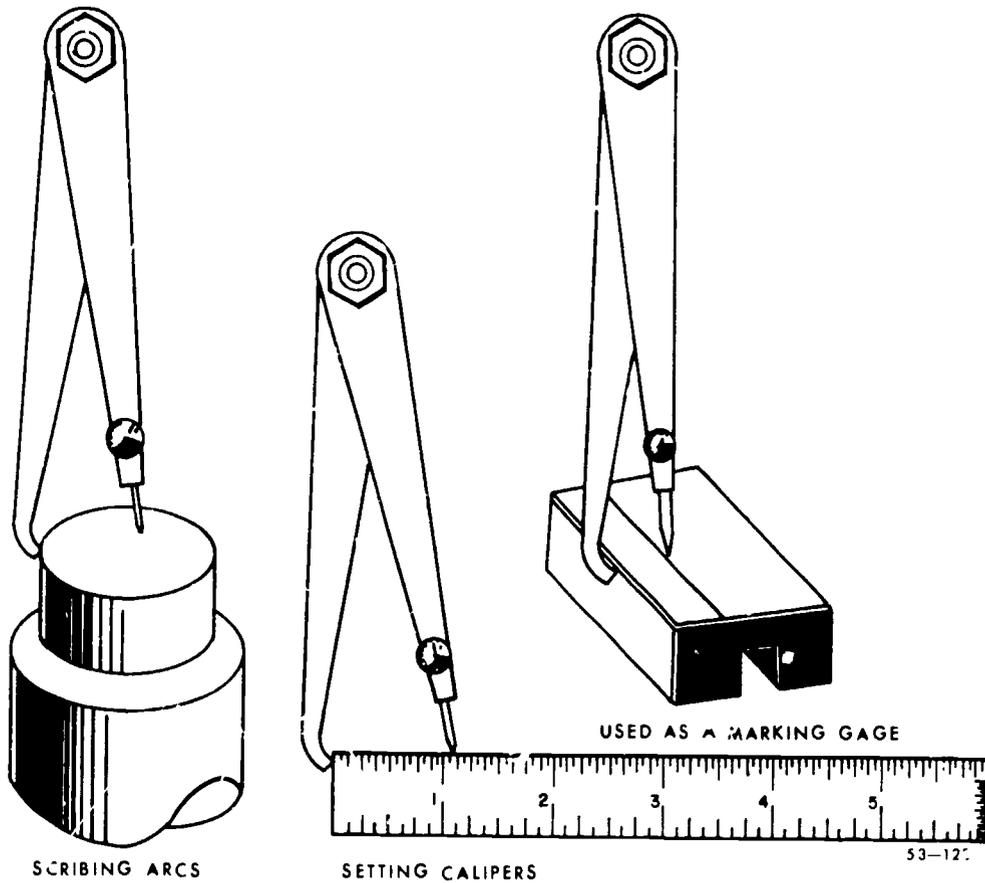
Figure 123. Using hermaphrodite calipers.
