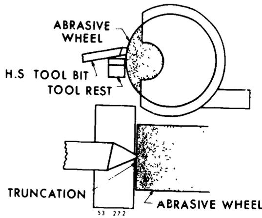
Figure 137. Grinding truncation.
