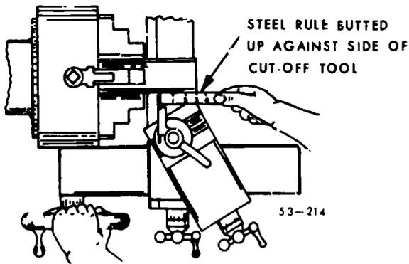
Figure 79. Measuring length to cut off.
