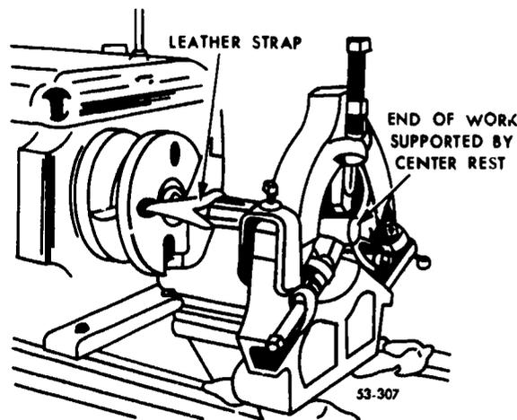
Figure 172. Tying the lathe dog.
