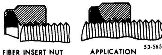
Figure 125. Fiber insert nut.
