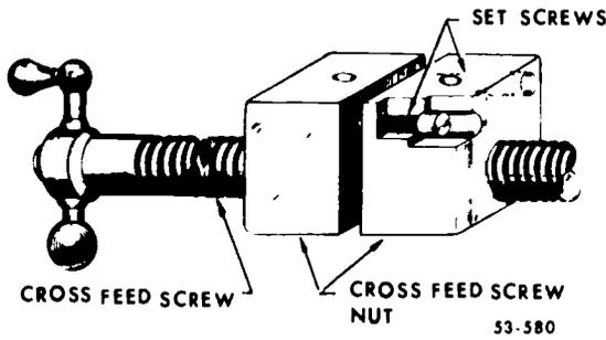
Figure 149. Crossfeed screw wear adjustment.
