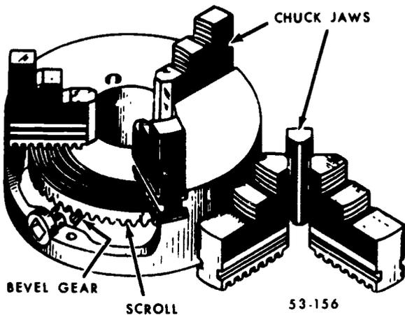
Figure 21. Three-jaw universal chuck.
