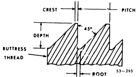
Figure 160 Buttress thread.
