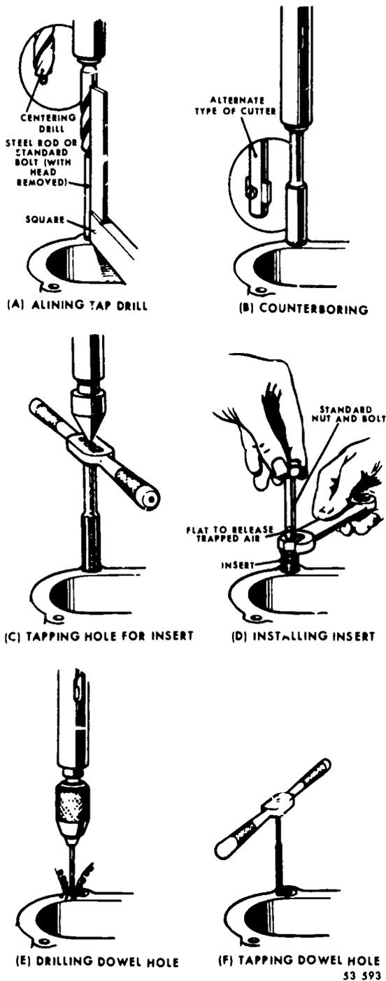
Figure 140. Installation of solid insert.
