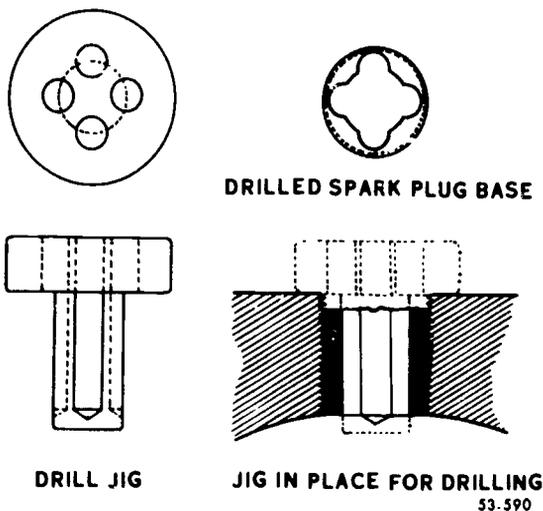
Figure 137. Spark plug drill jig.
