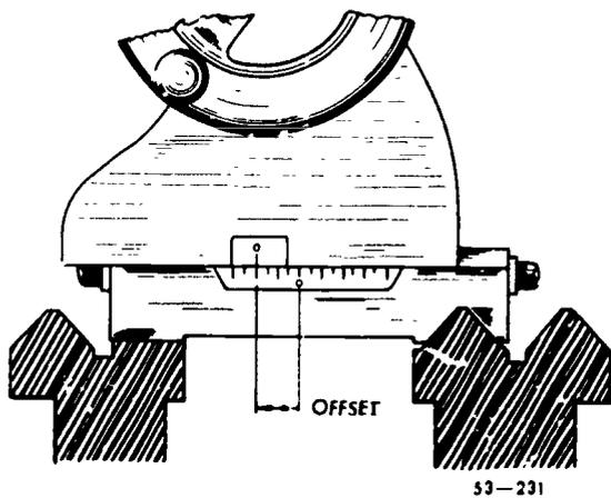
Figure 96. Tailstock cricket marks.
