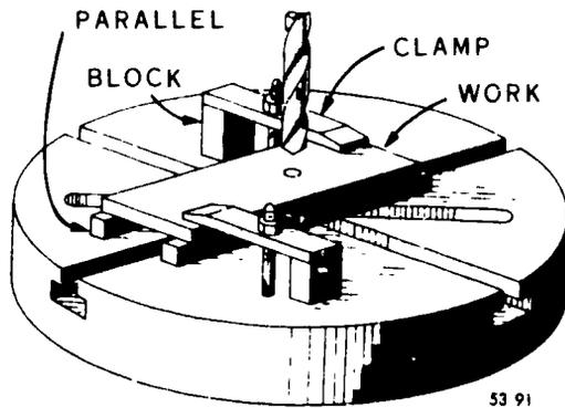
Figure 91. Work clamped to table.
