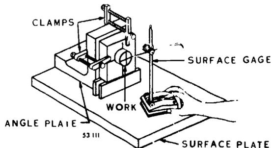
Figure 111. Use of angle plate in layout.
