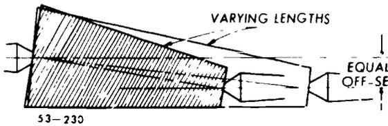
Figure 95. Effect of work length on taper.
