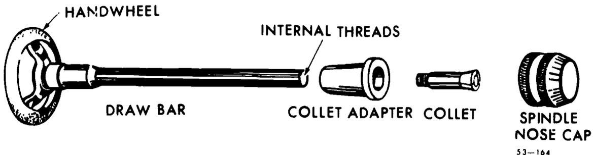
Figure 29. Draw-in collet chuck assembly.
