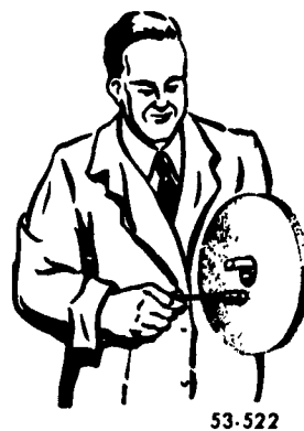
Figure 3-4 Checking for cracks
