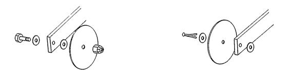
Assemble the wheel as shown, tightening the nut or bending the brad until the wheel rolls freely but does not wobble.
