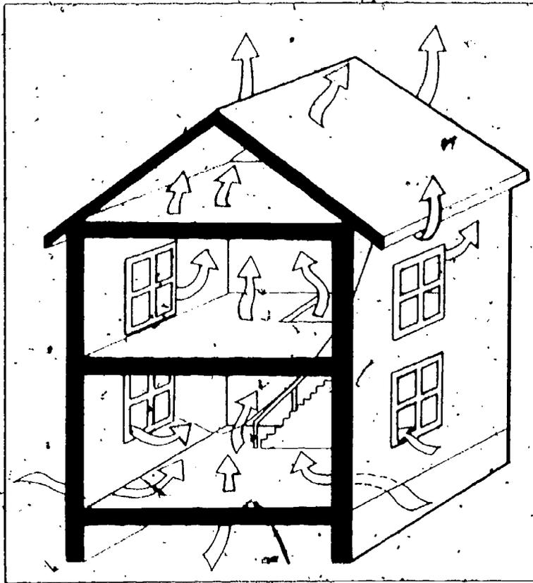
FIGURE 3: The "stack effect" is one significant way in which conventionally built houses lose heated air through infiltration and exfiltration.
