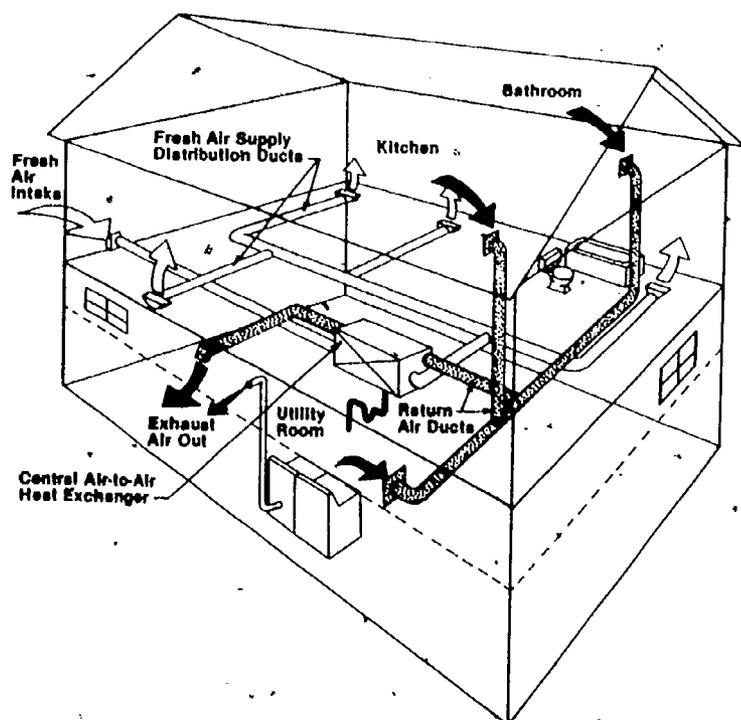
FIGURE 6: A fully ducted central air-to-air heat exchanger has the capability of distributing fresh air to and stale air from all areas of the house.
