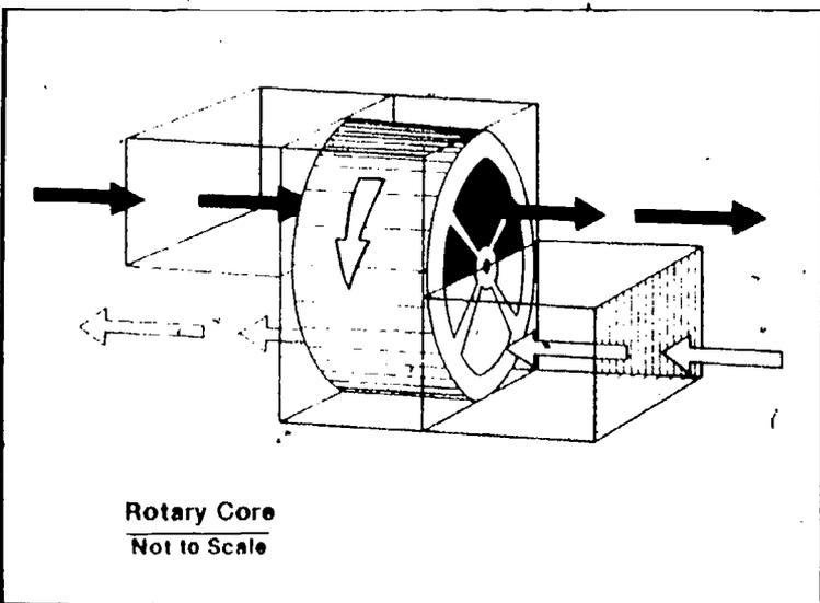
FIGURE 11: In rotary cores, a rotating wheel of tiny air passages transfers heat from one air stream to the other. Rotary cores usually transfer moisture as well as heat.
