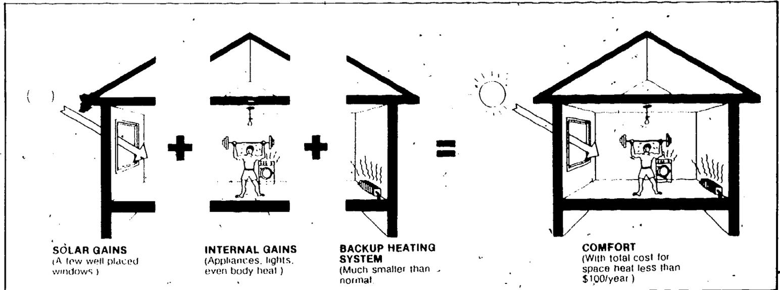
**FIGURE 1:** Superinsulation is a fast-growing trend in northern climates. Solar gains, internal gains from lights, appliances and occupants, and a small back-up heating system result in comfort at greatly reduced operating costs.
