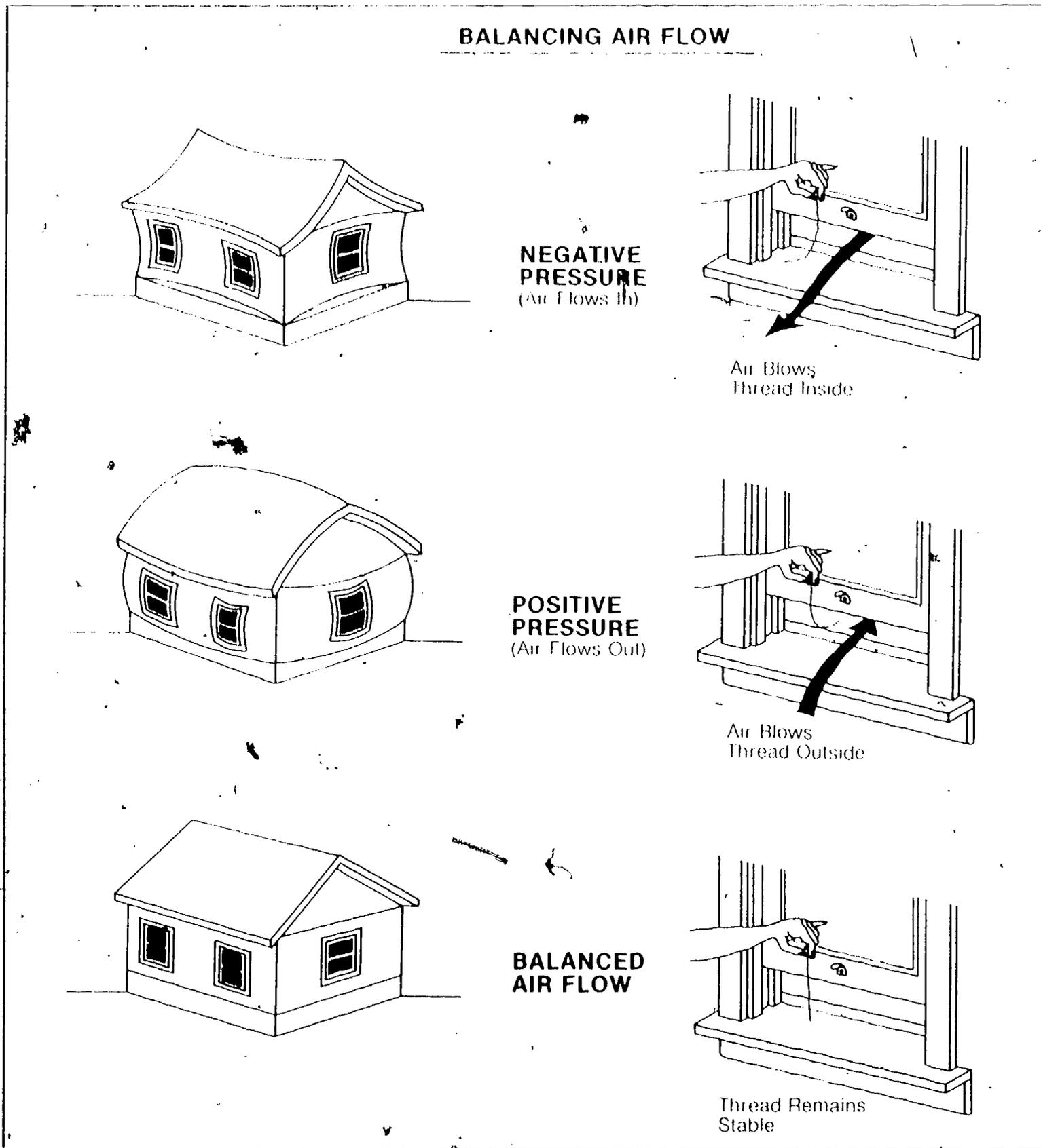
**FIGURE 16:** A balanced air flow is the goal when adjusting the heat exchanger's air intake and outflow levels. This can be accomplished by dampers. On a mild day with low wind speeds, the air flow can be balanced with a two-person check. One person observes whether air is leaving or entering the house, while the other person adjusts dampers until the flow is balanced. More sophisticated techniques are also available for use in this task.
