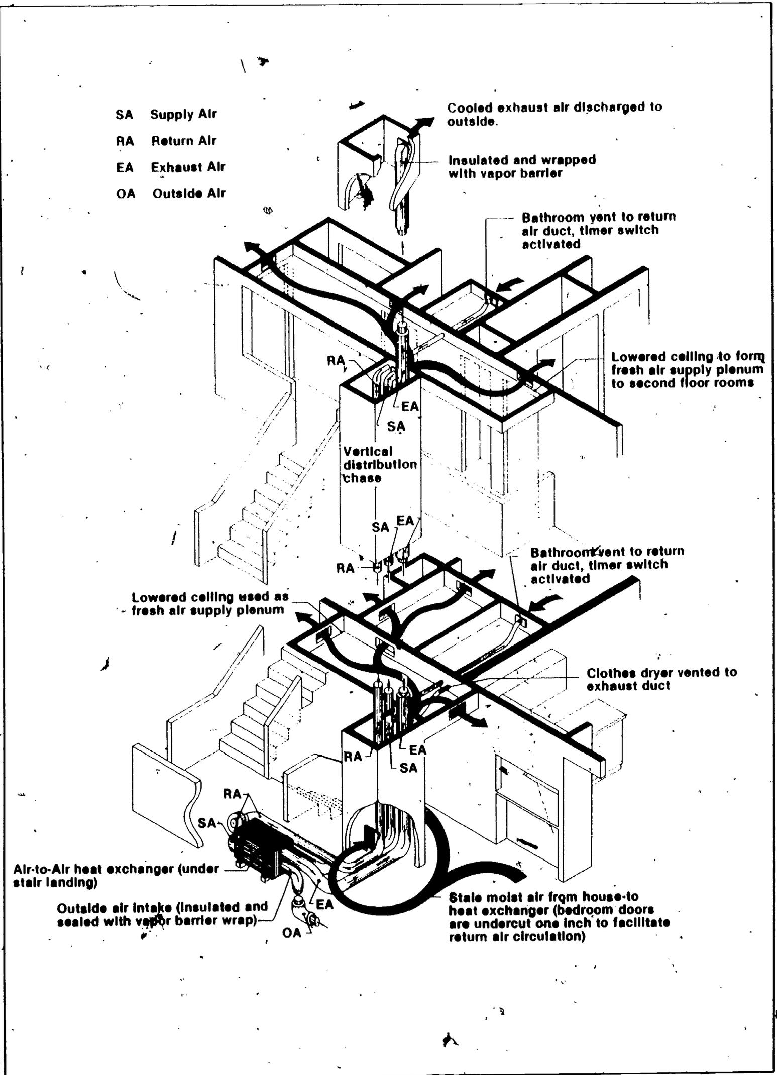
FIGURE 7: This isometric cutaway shows how the integration of a central, ducted air-to-air heat exchanger is best accomplished during the design phase. The system shown is for a two-story house.
