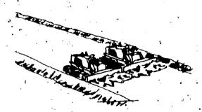
Fig 2-19. Blade-to-blade dozing.
