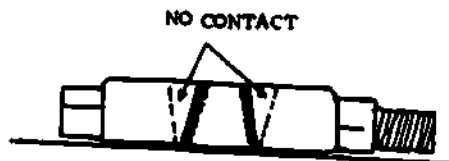
C. Clamp upside down will not make contact at top of post.
