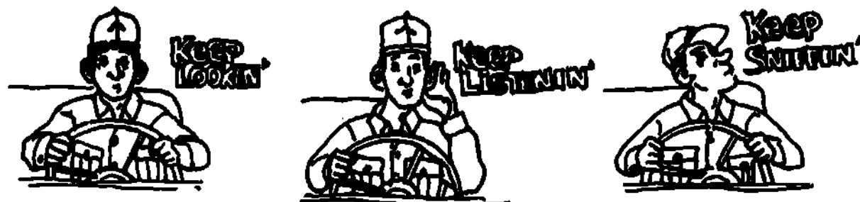
Fig 2-40. During-operation check--look, listen, and smell.
