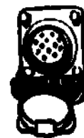
(14) Trailer coupling receptacle-Cap missing or sprung, male prongs don't make contact, dirty, outer ring damaged
