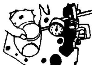
Fig 5-54. Measuring valve stem to valve guide clearance.
