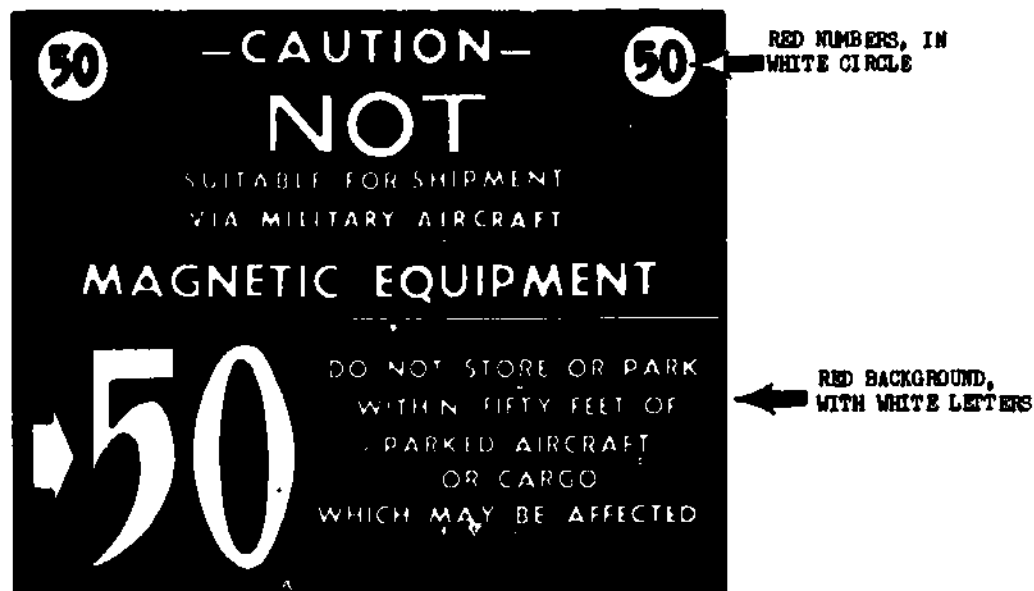
Fig 6-30. Caution label for magnetic equipment not suitable for air shipment.
