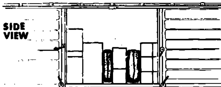
Fig 3-15. Pneumatic dunnage units staying load of various package sizes.
