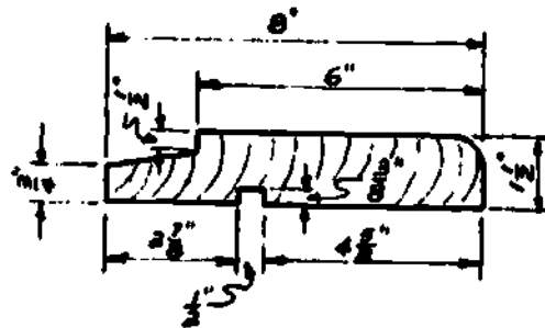
SLIDING DOOR SILL DETAIL SCALE: 3" = 1'-0"
