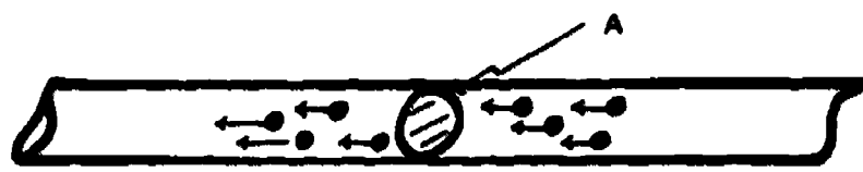
FIGURE A5-1 Electron Flow in a Wire
