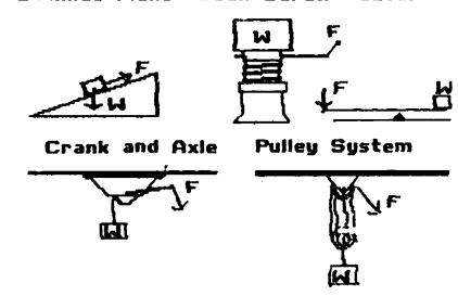
A MACHINE is any device by which the magnitude, direction, or method of application of a force is changed in order to achieve some advantage.
