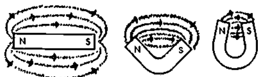
(8-22) FORMING A HORSESHOE MAGNET Courtesy of John Deere Ltd
