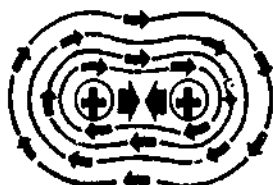
CONDUCTORS TEND TO MOVE TOGETHER
