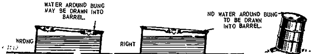
(5-50) STORAGE PRACTICES WHICH PREVENT CONTAMINATION OF OIL
