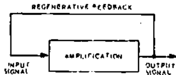
Figure 1-1. Basic Oscillator Block Diagram
