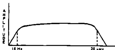
Figure 3-44. Frequency Response of Transformer-Coupled Audio Amplifier
