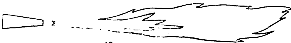
LP gas burning in atmosphere (Open fuel gas valve until flame begins to leave tip end.)
