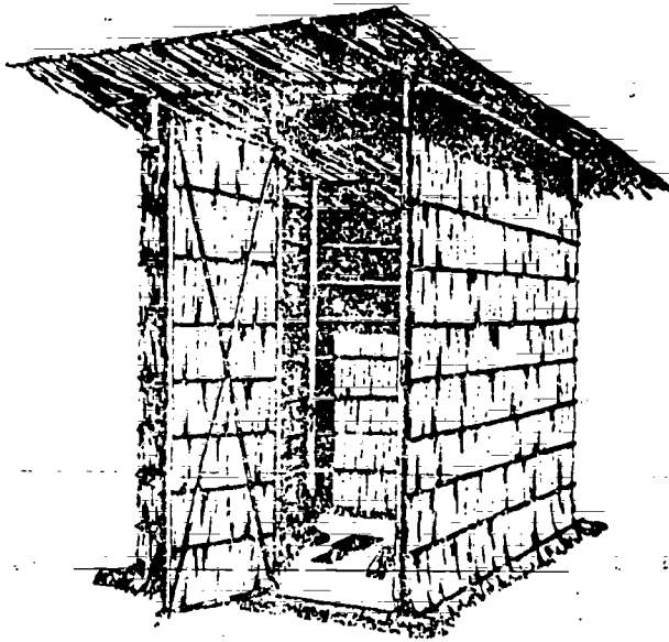
Fig. 67 Types of Privy Shelters COMPLETED PRIVY, SHOWING PALM THATCH WALL AND ROOF COVERING
