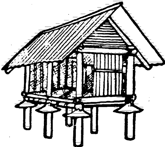
Fig. 53 Improved crib built from imported materials, Swaziland
