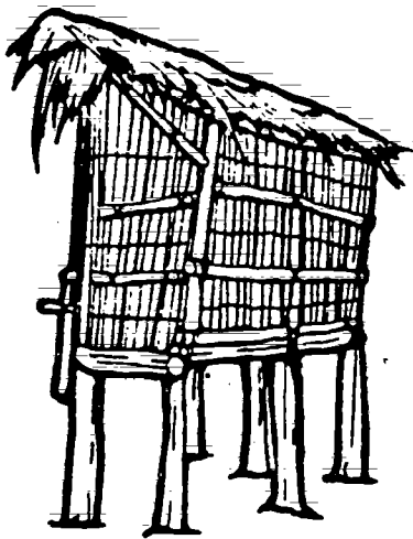
Fig. 41 Improved maize crib built from local materials
