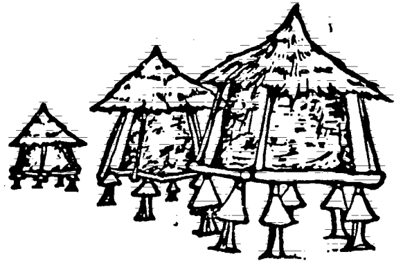
Fig. 50 Traditional nkhokwe improved with rat guards and muddying, Malawi
