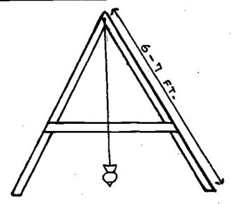
A. Build the A-frame as above using either lumber (1 x 2's or 2 x 2's) or poles cut from brush. Nails or twine can be used to hold it together. The cross-arm is placed about half-way up. The string with end weight should be hung from a nail placed midway in the juncture where the 2 legs meet.
