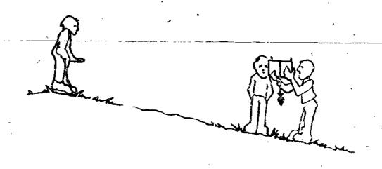
D. If the string rests on the  $84^{\circ}$  mark, then the actual slope angle is  $6^{\circ}$  (i.e.  $90^{\circ}$  -  $84^{\circ}$  =  $6^{\circ}$ ). Use the table on page 153 to convert degrees slope to percent slope.
