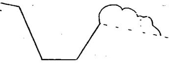
A live barrier (or use rocks) should be installed immediately above the uphill side of the ditch to prevent soil from filling it in. A live barrier should be about 12" (30 cms.) wide; a close growing grass like elephant; guinea, or jaragua works great; so does pineapple or sisal.
