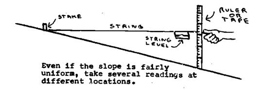
Sample Problem: Suppose your string is 400 centimeters long (4 meters) and that you measure a vertical drop of 36 centimeters. The slope would be:
