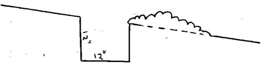
To prevent the ditches from eroding, the sides should then be tapered like so:
