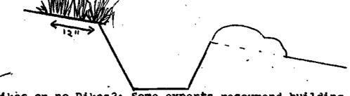
6. Dikes or no Dikes?: Some experts recommend building dikes every 5 meters (16') in the ditches to prevent excessive flow in the ditches. Others feel flow won't be excessive if the ditches don't slope more than 1%.
