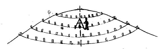
4. Even Out Irregularities: You don't want to end up with ditches full of zigs and zags, so try to smooth out any ragged portions by slightly altering the stakes.
