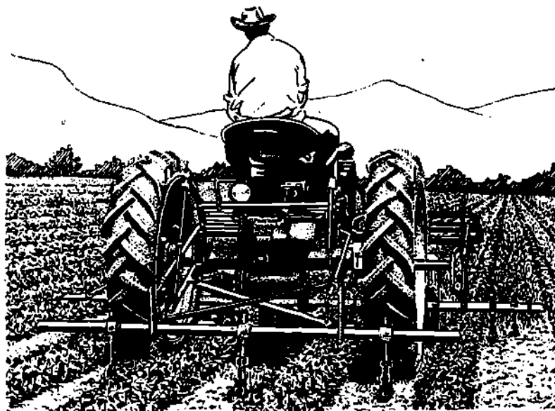
A tractor-drawn cultivator weeding beans . This particular model is mid-mounted , which allows the driver to view the weeding operation without having to turn around. Note the two outside shanks on the rear toolbar which help loosen the soil compacted by the tractor tires.
