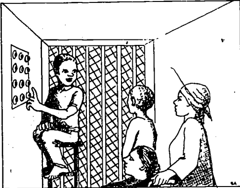
High position of control panel
