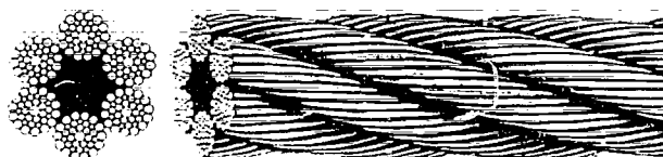
Figure 7-48. 6 x 36 Right Regular Lay, Fibre Core
