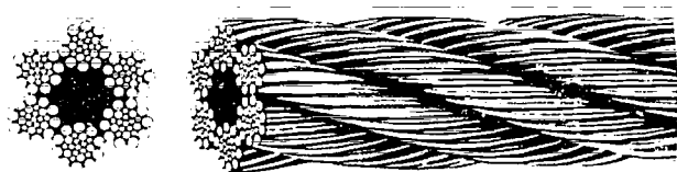
Figure 7-47. 6 x 26 Right Regular Lay, Fibre Core
