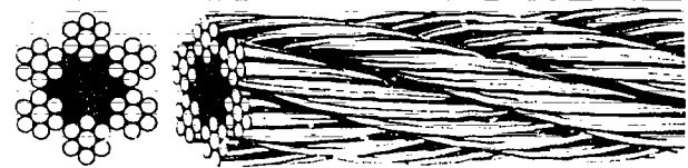
Figure 7-49. 6 x 7 Galvanized Right Regular Lay, Fibre Core
