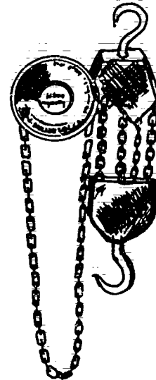
Figure 7-90. Chain Fall — Spur-Gear Hoist
