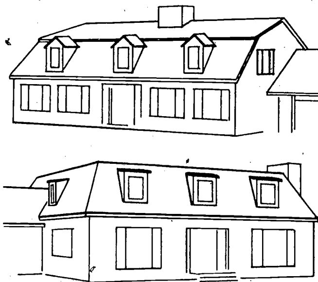
Fig. 9-2. Traditional roof designs. Above. Gambrel. Below. Mansard.
