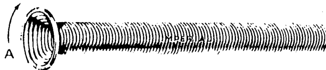
Tube bending spring may be fitted either outside or inside copper tube while bending tube. Bending spring reduces danger of flattening tube while it is being bent. A - Twist to remove spring.
