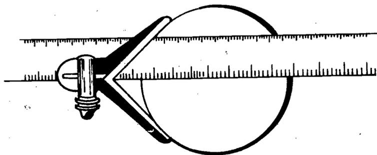
The Center Head speeds the measurement of diameters and improves reliability. For layout purposes the Center Head provides one of the most satisfactory methods for finding the centers of shafts.
