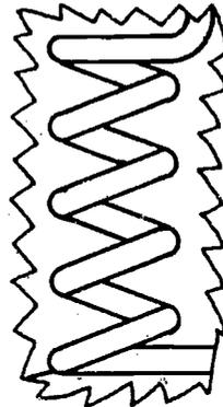
INTERNAL EXCHANGER (DRAIN BACK)
