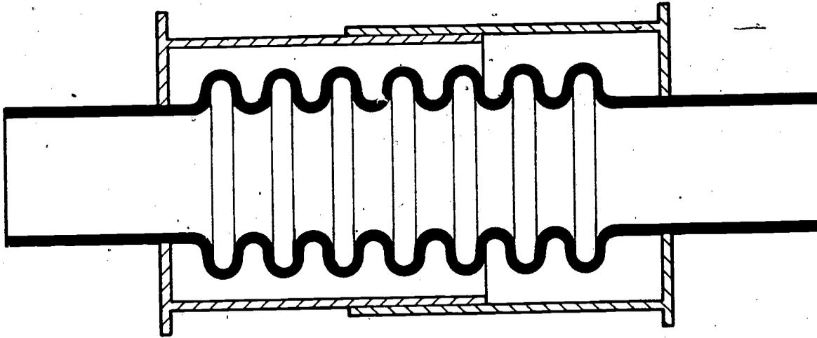
THERMAL EXPANSION/CONTRACTION COMPENSATOR
