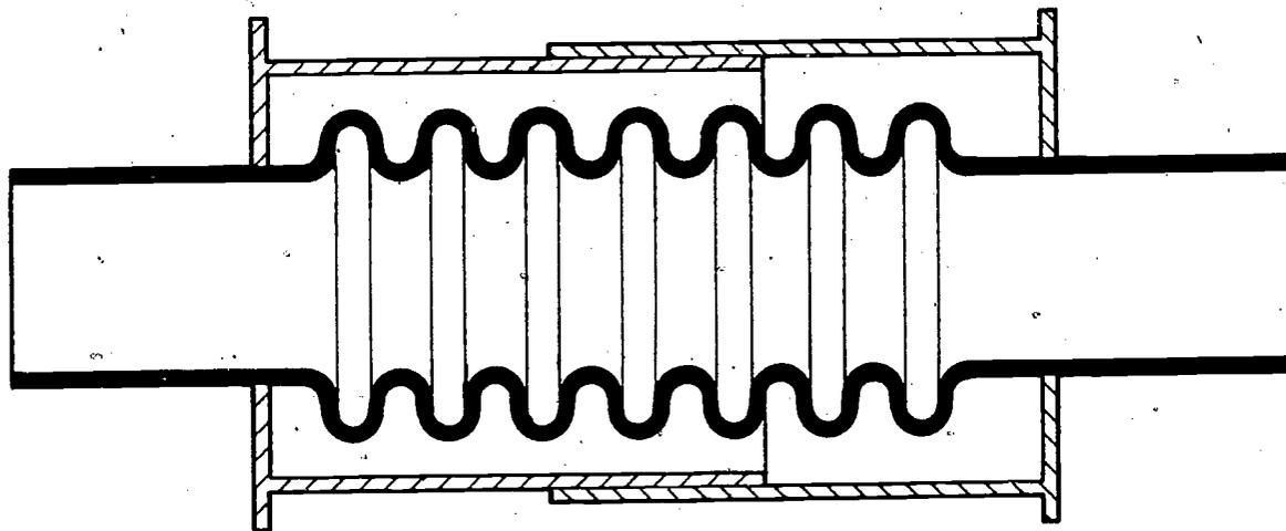
THERMAL EXPANSION/CONTRACTION COMPENSATOR
