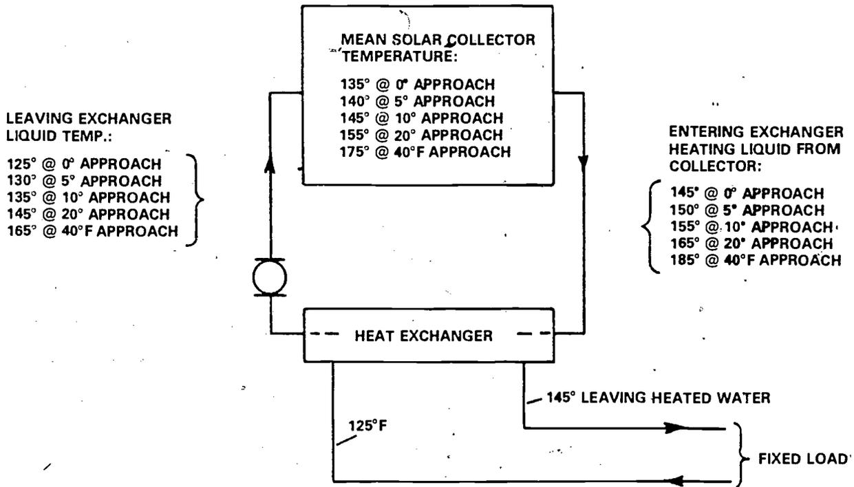
**CHANGE IN MEAN LIQUID TEMPERATURE IN SOLAR COLLECTORS WITH CHANGE IN HEAT EXCHANGER DESIGN APPROACH  $\Delta T$**
