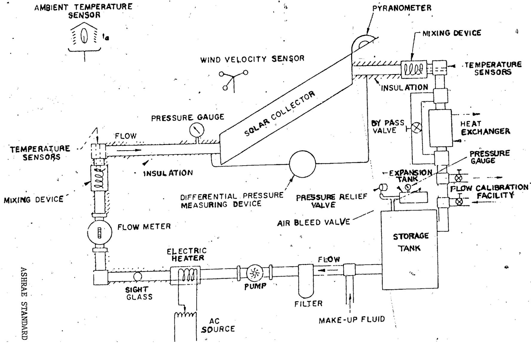
Fig. 1 Closed-Loop Testing Configuration for the Solar Collector when the Transfer Fluid is a Liquid
