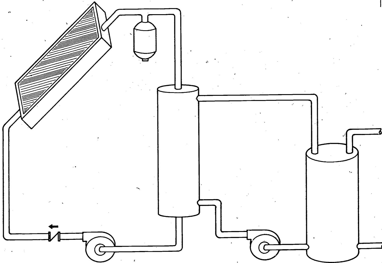
SYSTEM WITH SEPARATE HEAT EXCHANGER
