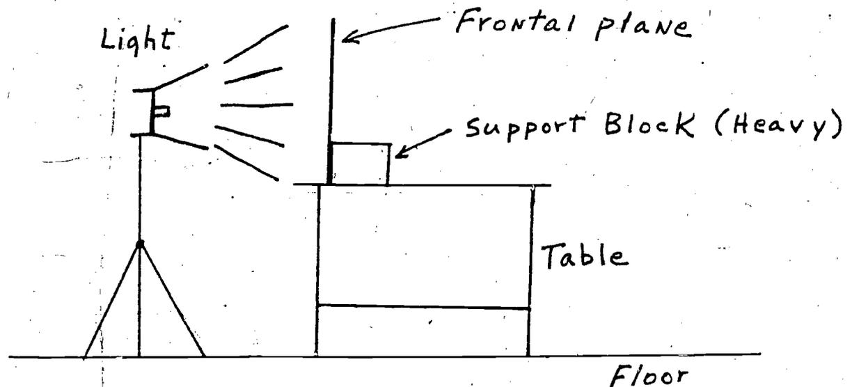
2. Place the light 1-3 feet from the frontal plane. Place a solar meter (Photo cell) scaled to measure  $\text{Btu/ft}^2/\text{hr.}$  and/or Langley's/hr. flush with the frontal plane.
