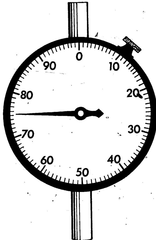
The spindle of a Dial Indicator is intended to work dry. It is important that it is never oiled or greased. The spindle is made a very close fit in its bearings and even thin oil will collect dirt which will cause the Indicator to stick.
