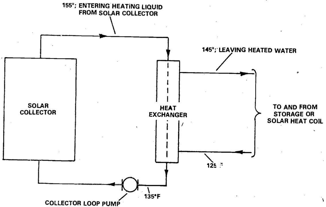
HEAT EXCHANGER DESIGNED FOR 10°
