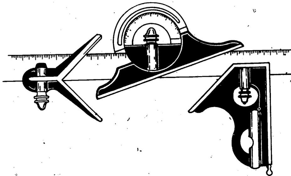
The Combination Square Set consists of a blade, protractor, center head, and a square head. This instrument combines all features of the center head, protractor, and square head. This versatile tool allows you to use one tool for layout assembly, inspection, and many other uses.
