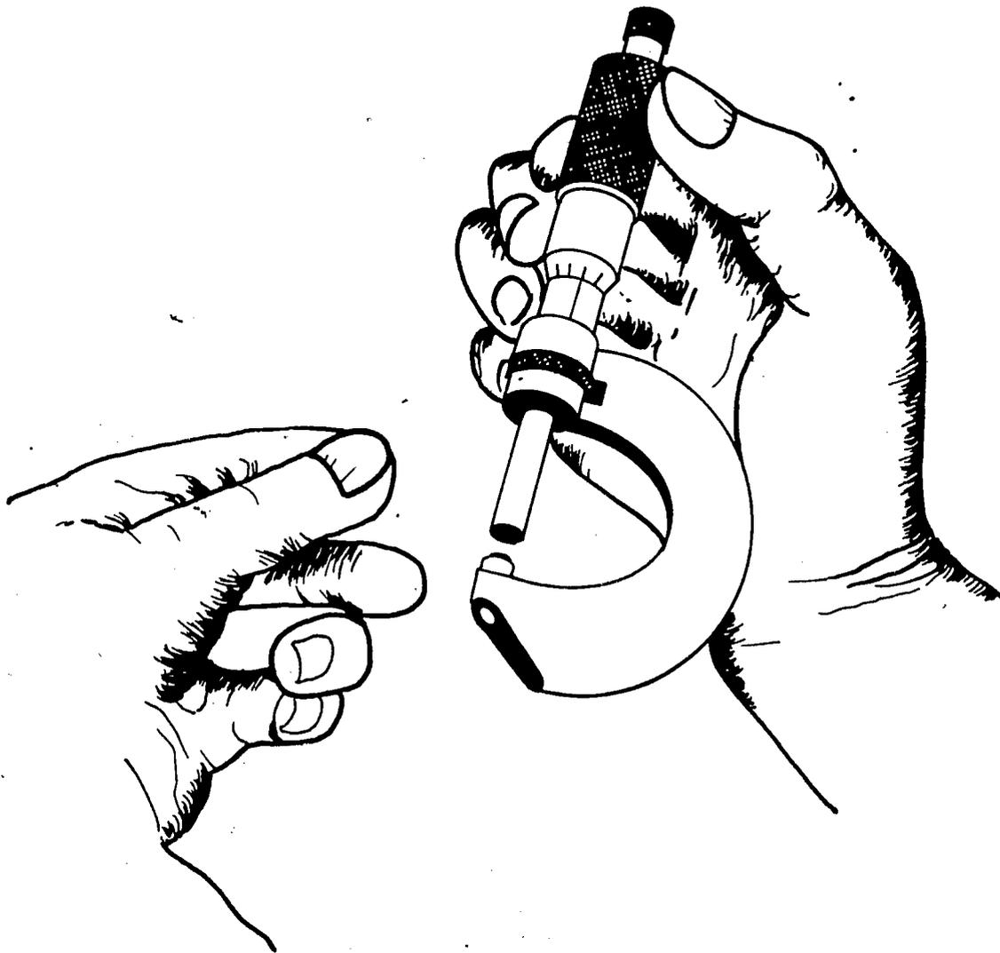
A handy method to clean the contact surfaces is to close the micrometer lightly on a piece of soft paper. It is then withdrawn. The paper will probably leave fuzz and lint on the surfaces. Blow this out with lung power - not the air hose. Never use compressed air to clean any precision instrument. The high velocity forces abrasive particles into the mechanism as well as away from it.
