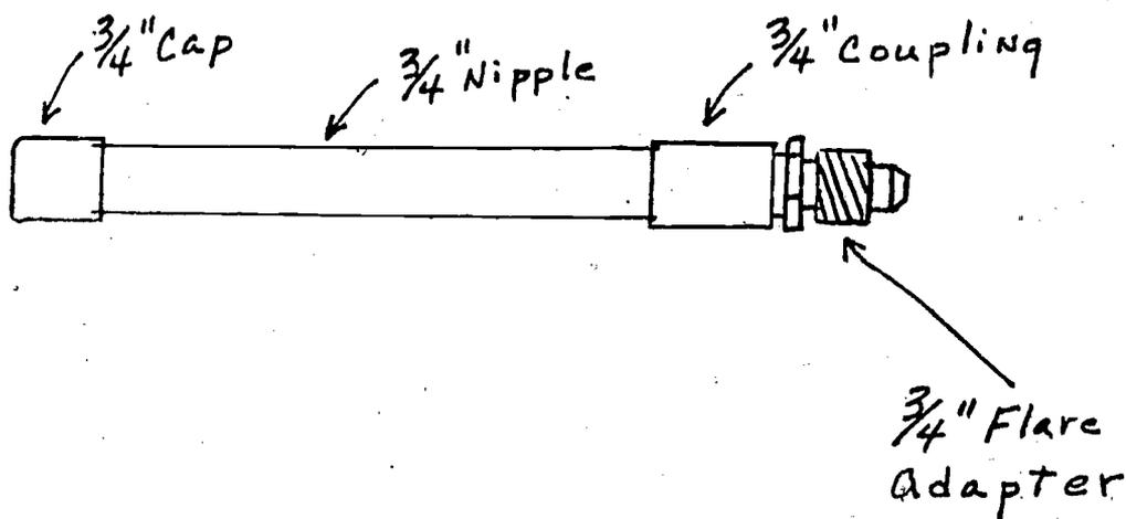
14. Pressure test the assembly using air or refrigerant.
