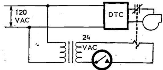
2. Simulate freezing conditions by placing the thermal switch in an ice bath. Protect the switch from moisture with a plastic bag.
