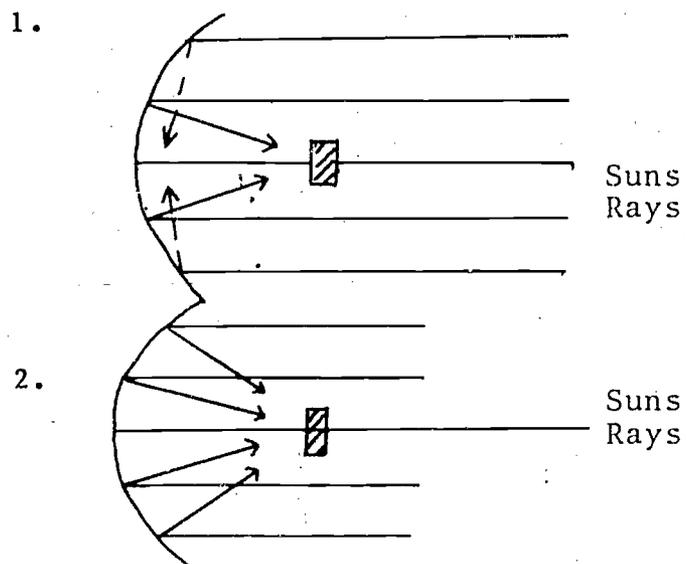
All rays incident on reflector parallel to principal axis will reflect on to absorber.
