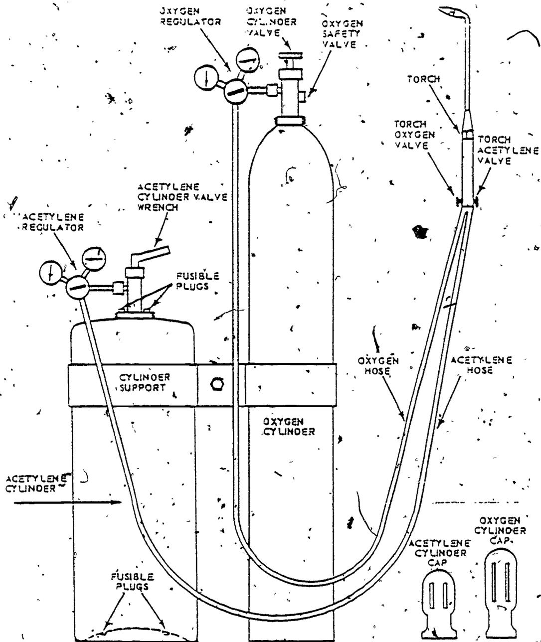
An oxygen-acetylene welding outfit.
