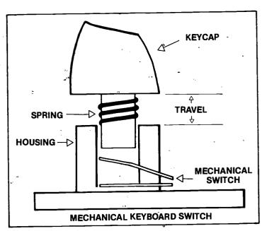
Mechanical Switch: This is the least expensive of switch devices and uses a plunger type mechanism which results in a metal to metal contact. Life cycle of 8-10 million cycles.
