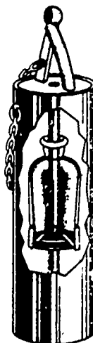
Figure 7. Device for Taking Dissolved Oxygen Samples
