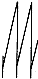
A TRAPEZOIDAL WAVEFORM INCORRECTLY PROPORTIONED; VERTICAL GAIN HIGH, HORIZONTAL GAIN LOW
