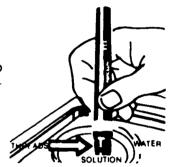
B. Blot the cleaning solution from the air channel with a paper wipe
