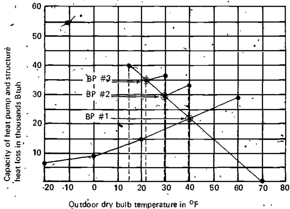
Plotting balance points indicates a need for 8-kw of supplementary heat; 4-kw would be energized in the first two heating stages by the indoor thermostat at BP #1, 2-kw would be energized by the first outdoor thermostat at BP #2, and the final 2-kw would be energized by the second outdoor thermostat at BP #3, and the unit is well balanced for both heating and cooling
