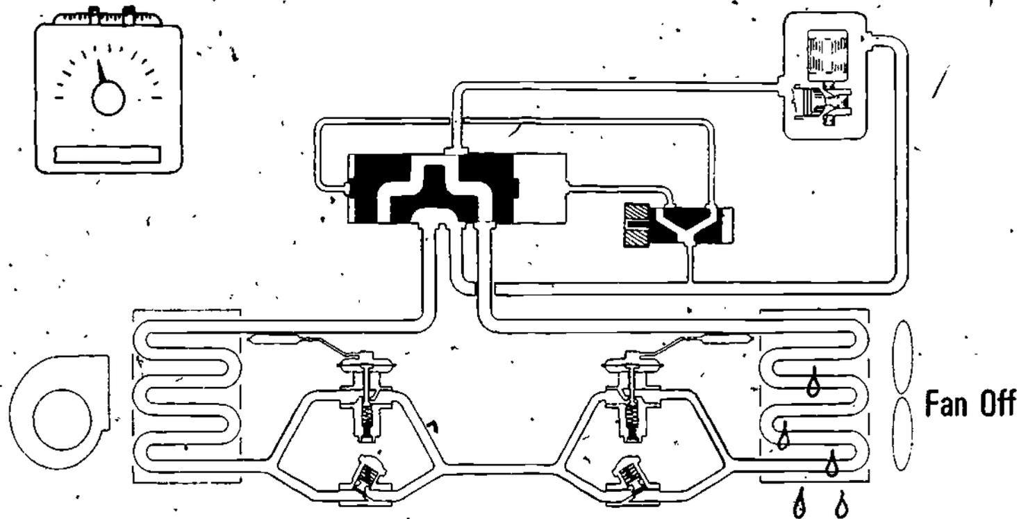
Ice Is Melted Off Coil
