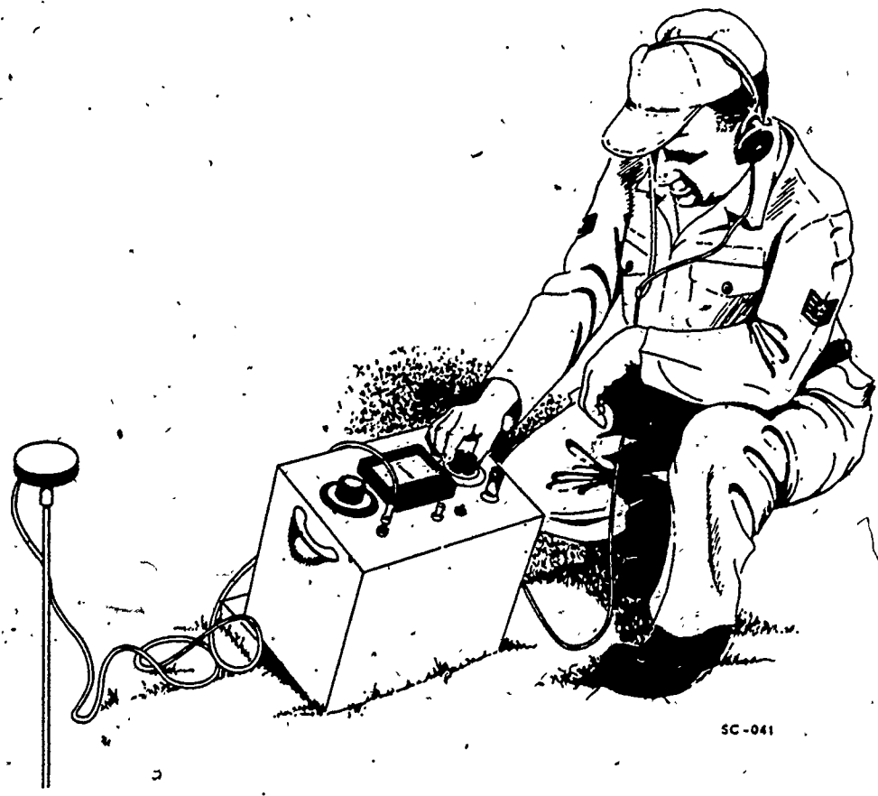
Figure 59. Using Microphone and Prodding Rod to Locate Leaks by Sound
