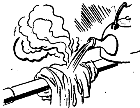
Figure 1. Hot Water Applied to Outside of Frozen Pipe
