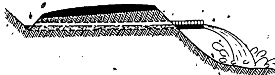
Figure 4-8. Culvert extended beyond fill to prevent erosion.
